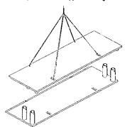
Set matching panet over bottom panet. Install Spreader pipes in collars and insert pins and keepers.
