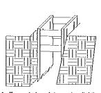
Excavate trench to grade, slightly wider than shield. Lift and tower shield into trench.
