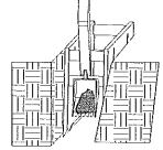
Perform desired work, then excavate in front of shield.
