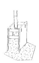
Excavate until soil begins to crumble beyond desired trench width, Place shield on line of excavation and excavate from within.
