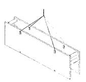
Place sling in top 4 lift lugs. Stand shield and install into trench.
