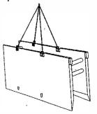
5. Place sling in top 4 lift lugs. Stand shield and install into trench.
