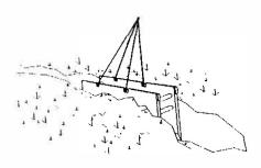
6. WARNING: Lift eyes are designed and intended for assembly and lifting only. Do not pull or lift by eyes when shied is stuck or has pressure against it. Loosen shield by pulling on spreader bars or digging along sides before using lift eyes.
