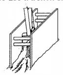
Excavate until soil begins to crumble beyond desired trench width. Place shield on line of excavation and excavate from within.
