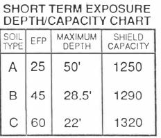
Shield capacity is in PSF per foot along the bottom of the Trench Shield
