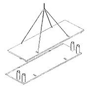
4. Set matching panel over bottom panel. Install Spreader pipes in collars and insert pins and keepers.
