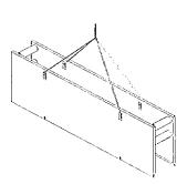
Place sling in top 4 lift lugs. Stand shield and install into trench.
