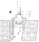
3. Pull shield forward by front spreaders or pulling eyes. Continue excavating and pull shield forward. Back fill as work progresses.
