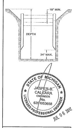
2" DIAM. PINS SHALL HAVE MIN Fu = 100 KSI. CONTRACTOR RESPONSIBLE FOR ENSURING PROPER GRADE PINS ARE IN PLACE PRIOR TO SHIELD USE.
