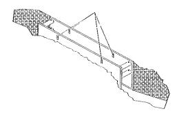
WARNING: Lift eyes are designed and intended for assembly and lifting only. Do not pull or lift by eyes when shleld is stuck or has pressure against it. Loosen shletd by pulling on spreader or digging along sides before using lift eyes.
