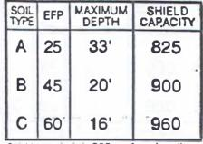
Shield capacity is in PSF per foot along the bottom of the Trench Shield
