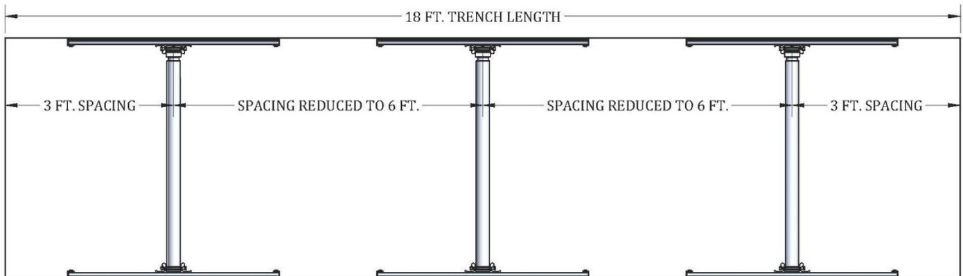
TRENCHES IN LENGTH GREATER THAN DOUBLE THE MAX HORIZONTAL SPACING, (18 FT.) IN THIS CASE WILL NEED THREE SHORES MINIMUM.
