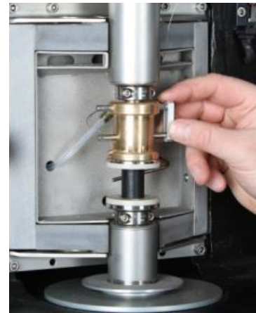
Specimen holder dedicated to HBU testing
