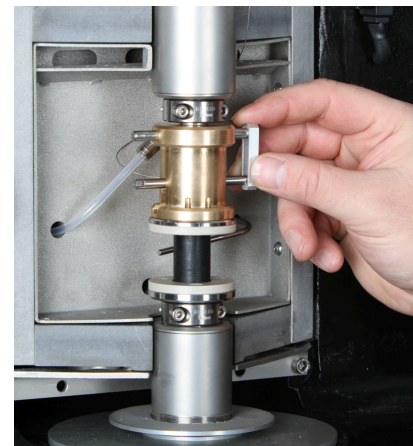
Figure 3. Heat build-up module (HBU)
