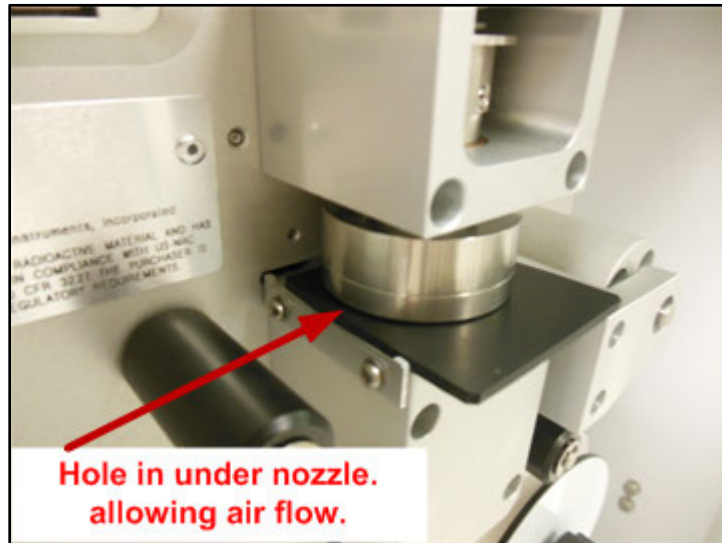
Figure 7-7 Nozzle Seal Tool, Total System Leak test
