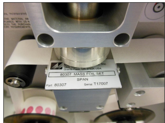
Figure 7-16 Span Foil Installed Above Tape
