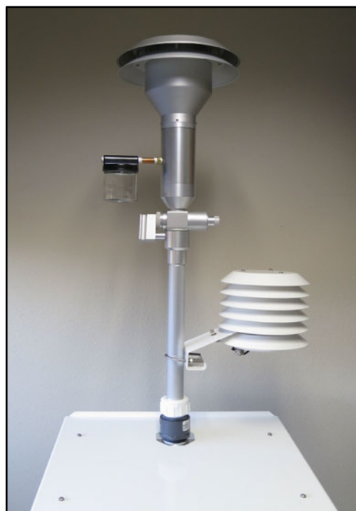
Figure 4-18 BX-802 and Cyclone Installed
