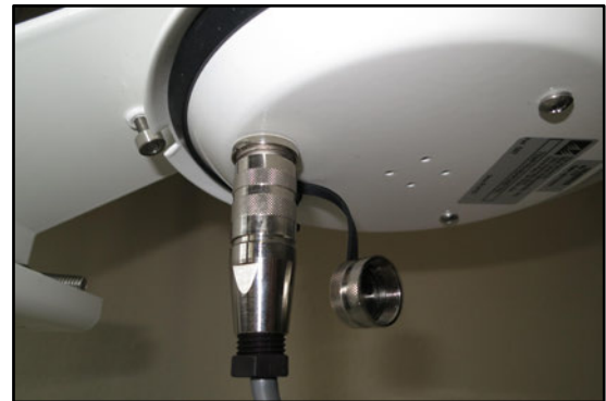
Figure 4-15 BX-597A Sensor and Cable
