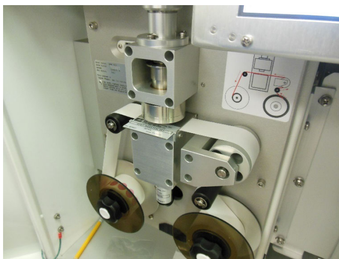
Figure 7-11 Span Foil Installed
