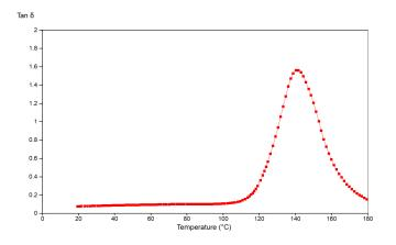
Figure 5. PMMA Tan  $\delta$  as a function of the temperature (from 20°C to 180°C) at 1 Hz.
