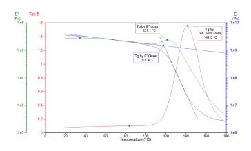
Figure 6. PMMA E', E'' and Tan δ as a function of the temperature (from 20°C to 180°C) at 1 Hz. Different ways to measure the Tg are highlighted.
