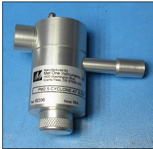
Figure 6-4 Unscrew and Clean Particle Trap
