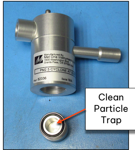
Figure 6-4 Unscrew and Clean Particle Trap
