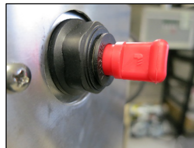
Figure 6-16 Leak Check Sealing Plug Installation
