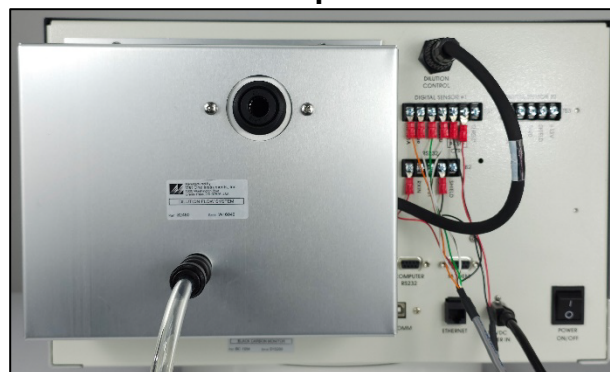
Figure 2-10 Dilution Flow System Installed
