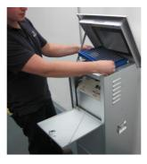
Figure 30 – Installing the loaded filter cassette
