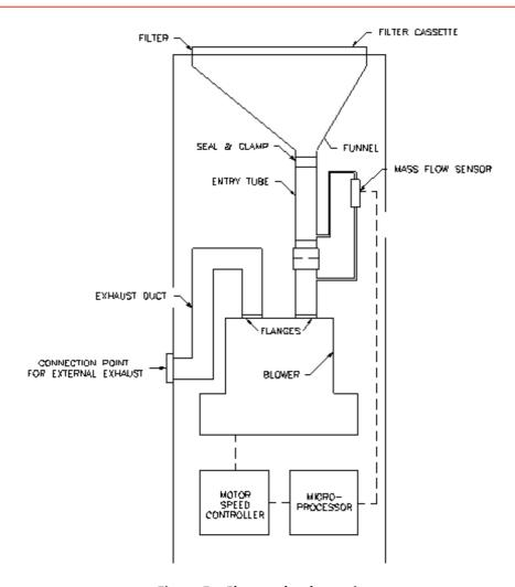
Figure 5 – Flow path schematic
