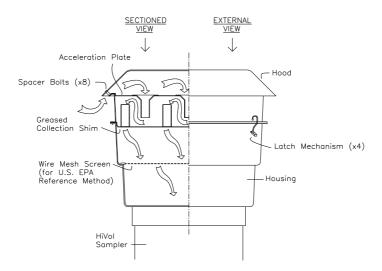
Figure 4 – Cross-section of PM<sub>10</sub> size selective inlet hood
