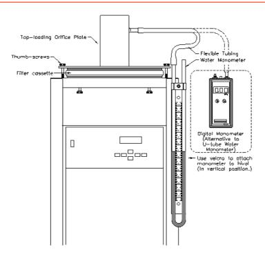
Figure 35 – Calibration set-up
