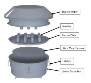
Figure 15 – PM<sub>10</sub> Components Layout
