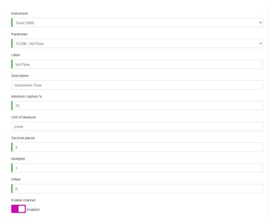
Figure 49 - Channel Setup
