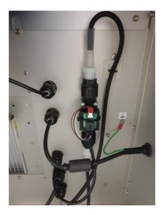
Figure 53 - Flow sensor
