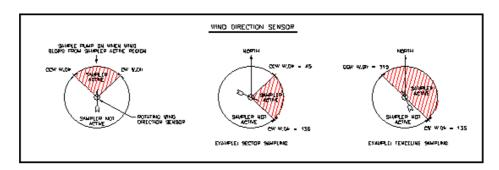
Figure 34 – Conditional sampling and wind direction sensor set-up
