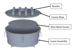
Figure 17 - Mesh and Inlet Inspection
