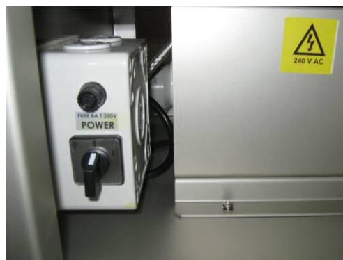
Figure 12 – Power switch location
