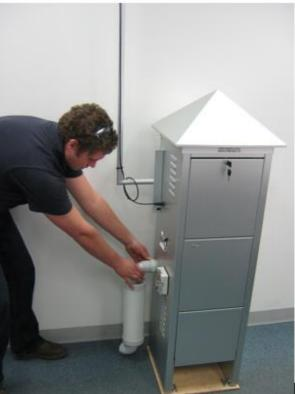
Figure 26 - Installing the optional muffler
