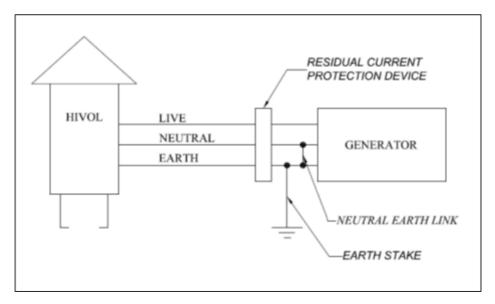
Figure 29 - HiVol Power Connection Using a Generator
