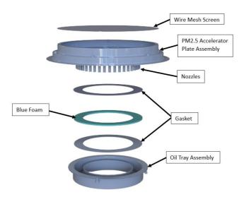
Figure 20 - Inspection Wire Mesh Screen and Inlet Nozzles
