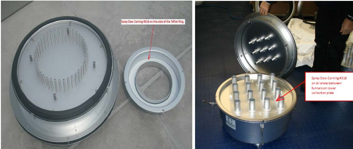
Figure 18 – Application of grease
