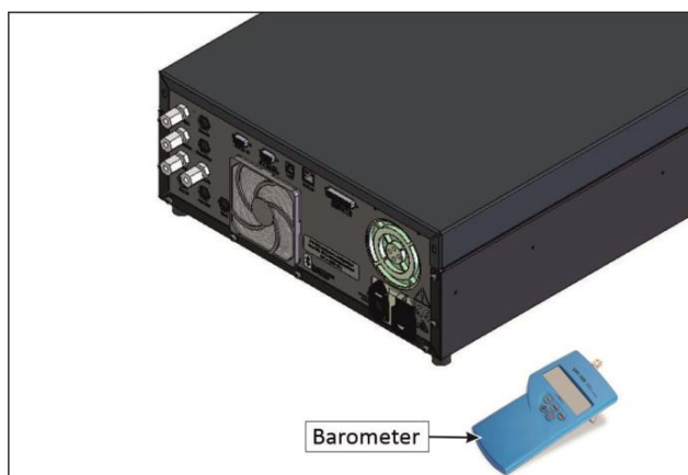
Figure 107 – Full Pressure Calibration Set-up (Ambient)
