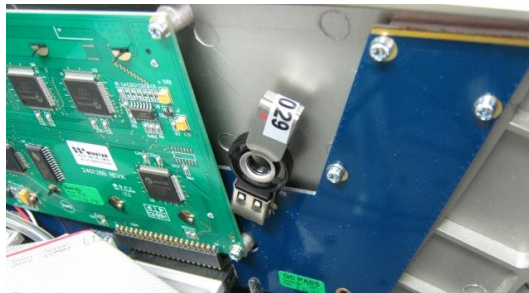
Figure 32 – Installation of USB Memory Stick
