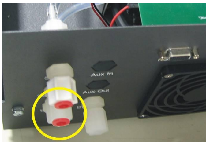
Figure 24 Plugged sample and calibration ports
