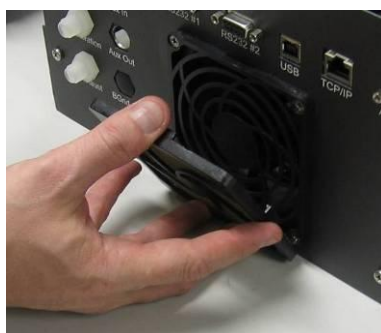
Figure 23 Removing fan filter
