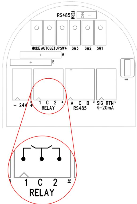
Figure 12: Connecting Relays
