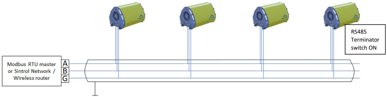
Figure 15: Connecting a RS485 Network
