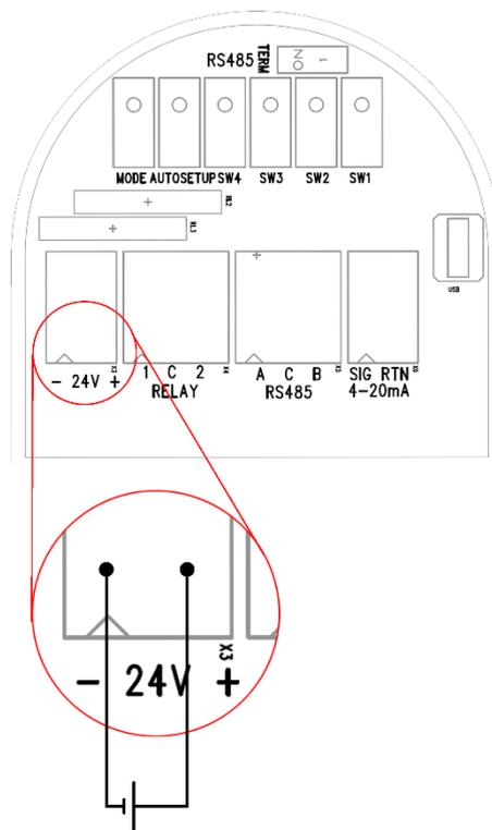
Figure 11: Connecting power input
