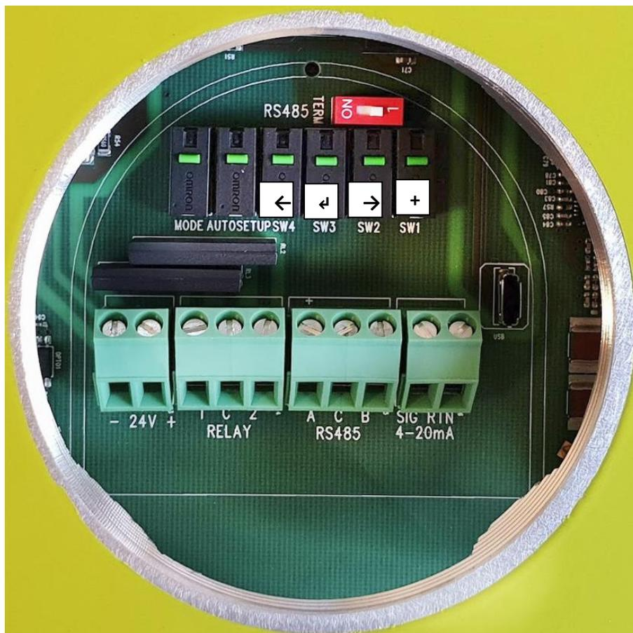
Figure 18: Bottom view of buttons
