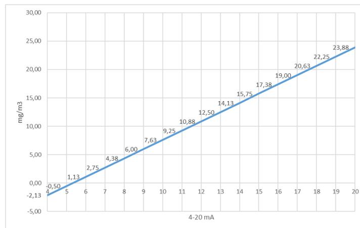
Figure 19: Example for display calibration
