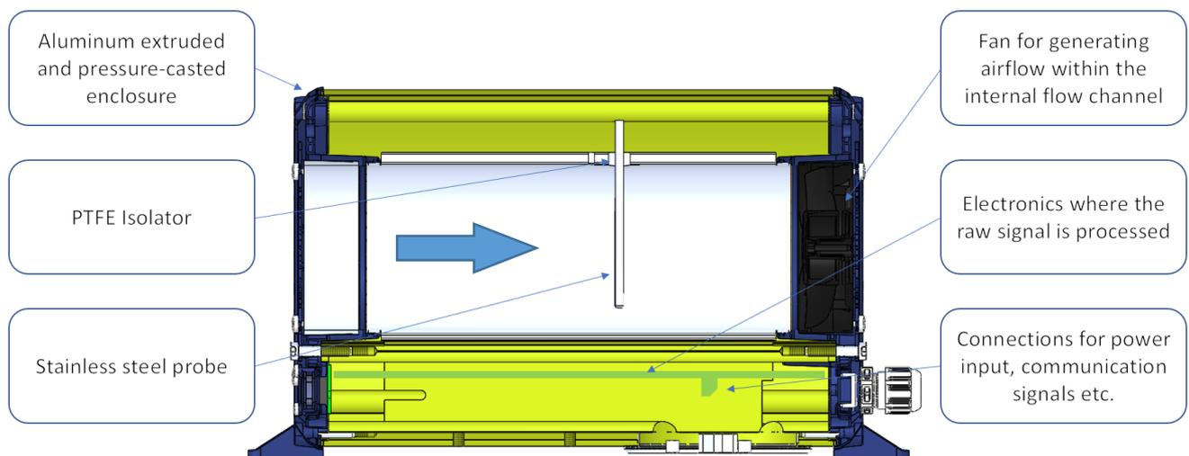
Figure 1 Dumo structure and main parts
