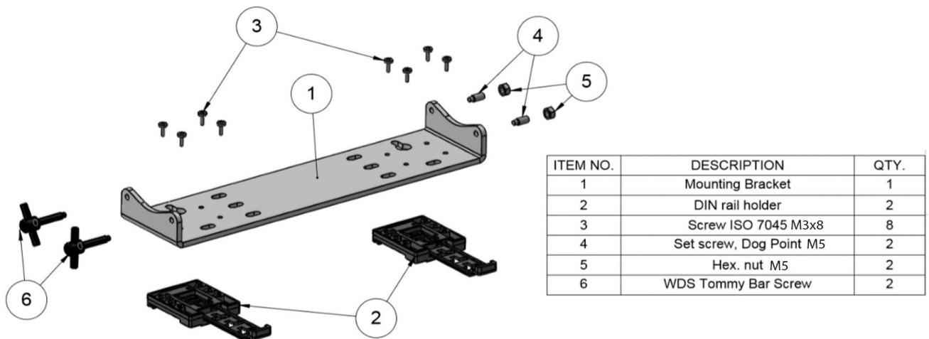
Figure 3 Wall/Din-rail mounting bracket
