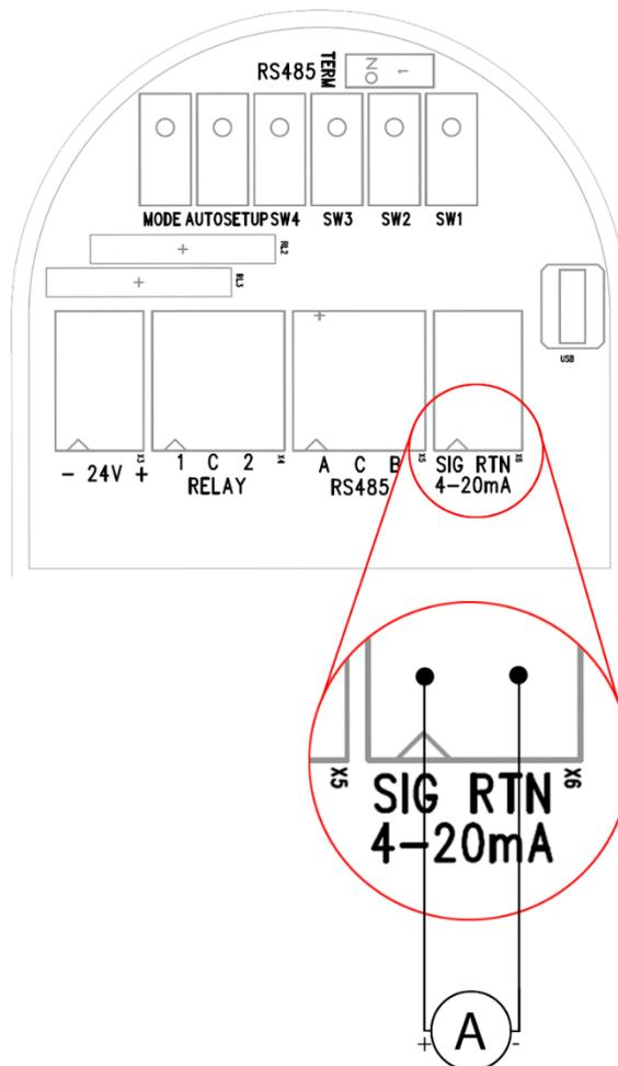
Figure 13: mA loop connection
