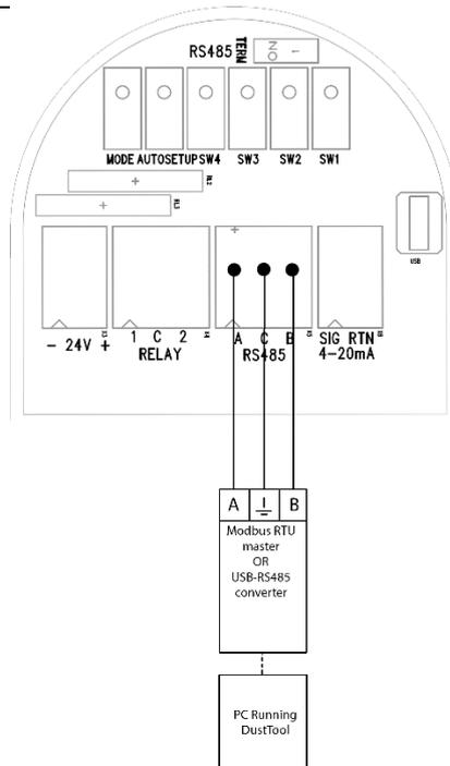
Figure 14: RS485 connections
