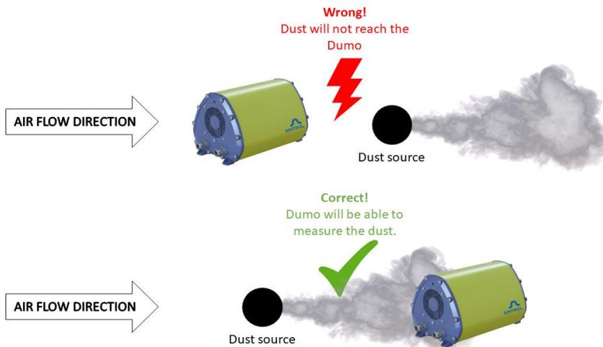
Figure 9: Installation Point in terms of air flow
