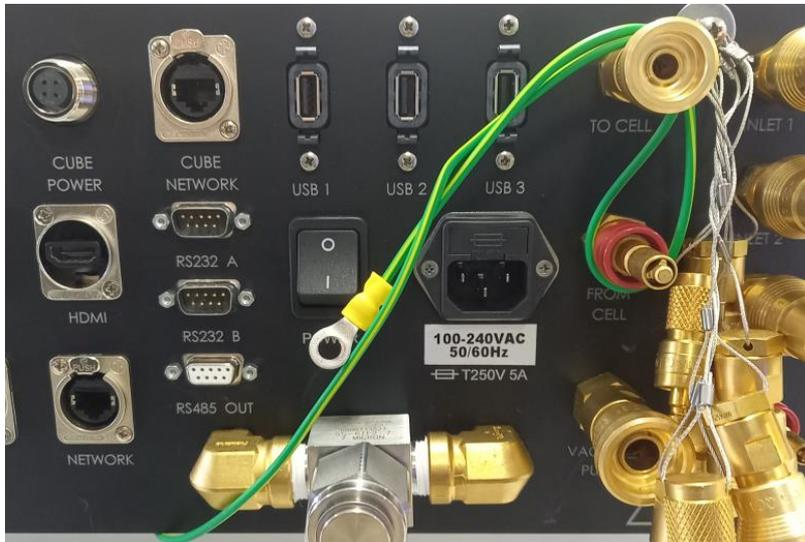
Figure 36 – Temporarily Position Earth Strap
