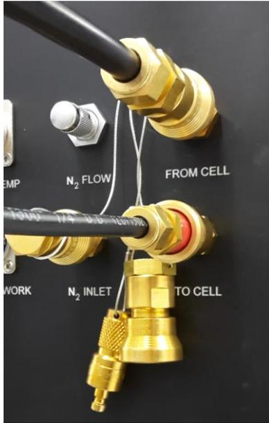
Figure 13 – Link Tubing - Optical Module
