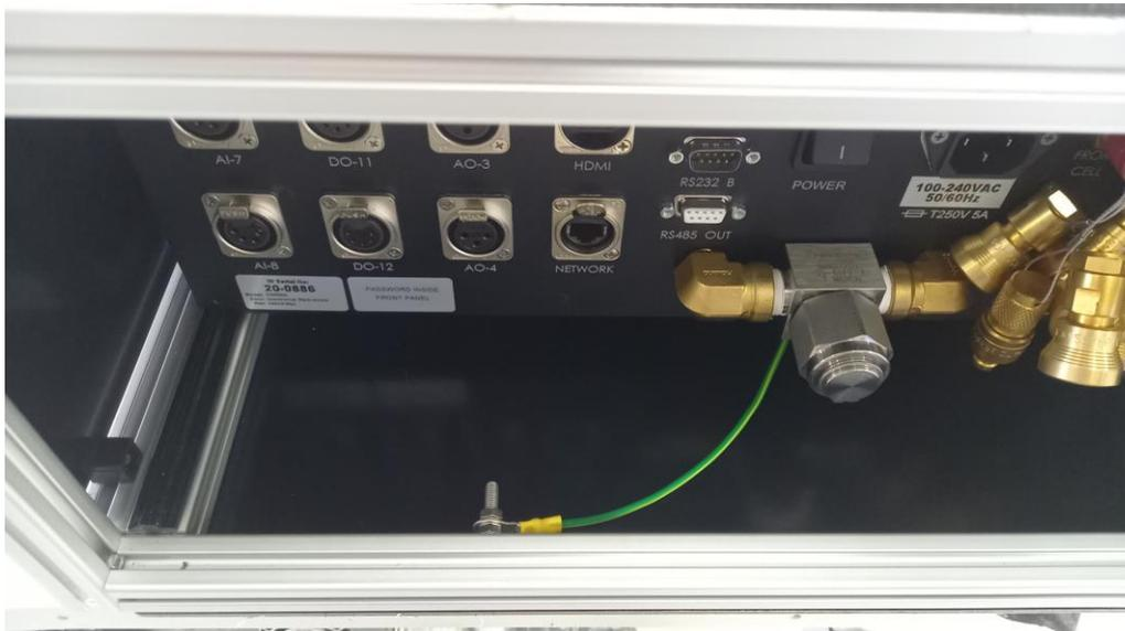
**Figure 32 – Location of the Earth Strap on the Auxiliary Module**
