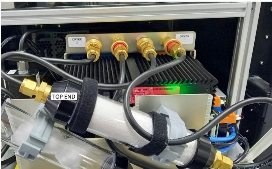
**Figure 9 – Dryer1 Quick Release Fittings**
