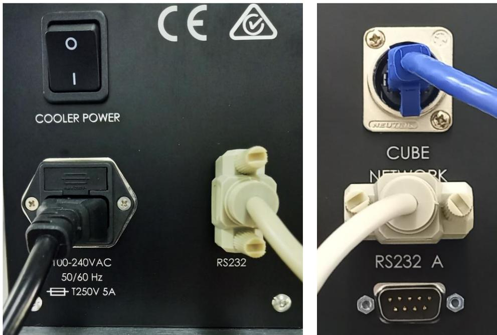
Figure 14 – TE Cooler to Auxiliary module RS232 link
