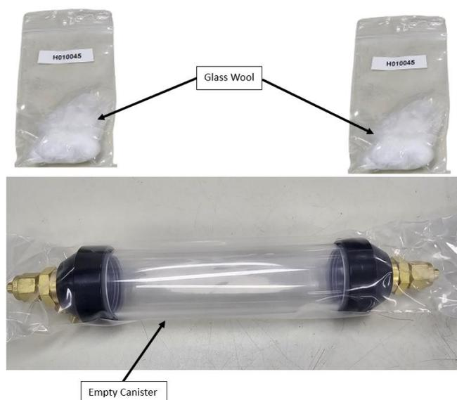
**Figure 10 – Empty Canister and Glass Wool**
