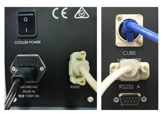
Figure 14 – TE Cooler to Auxiliary module RS232 link
