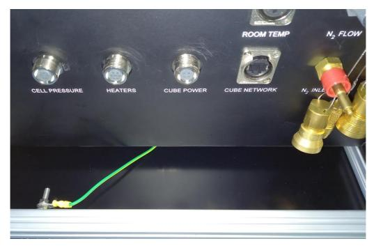
Figure 33 – Location of the Earth Strap on the Optical Module
