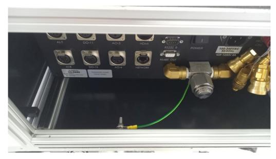
Figure 32 – Location of the Earth Strap on the Auxiliary Module
