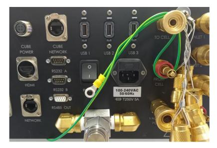
Figure 36 - Temporarily Position Earth Strap
