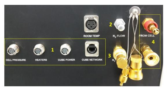
Figure 18 – Optical Module Connections
