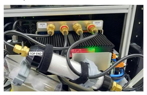
Figure 9 - Dryer1 Quick Release Fittings
