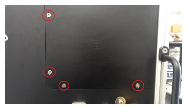
Figure 30 - Optical Module Rear Access panel (TE Cooler option)
