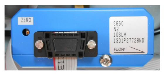
Figure 40 - MFC Zero Adjust Pot
