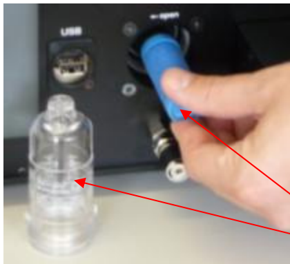
Fig. 38: Removing the filter
