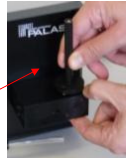
Fig. 33: Removing the cuvette
