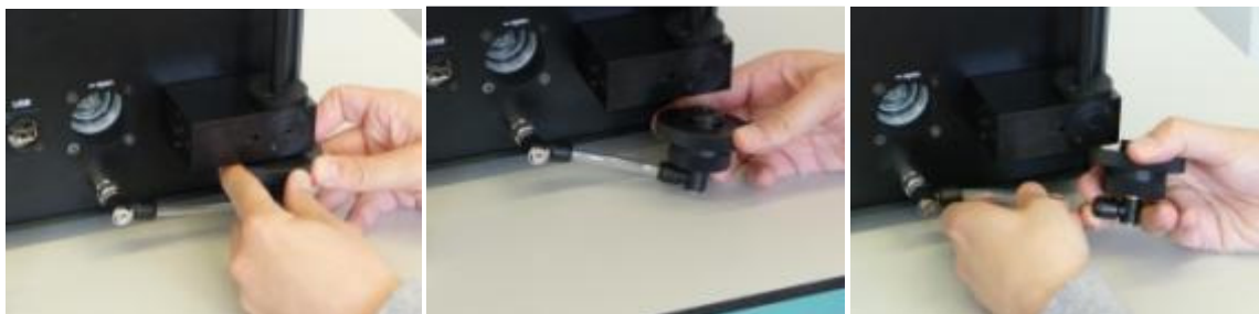
Fig. 31 A-C: Removing the filter holder
