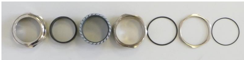
Fig. 7: Components of the fixing of the weather station tube
