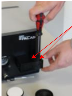
Fig. 32: Loosening the M3 cross-head screws
