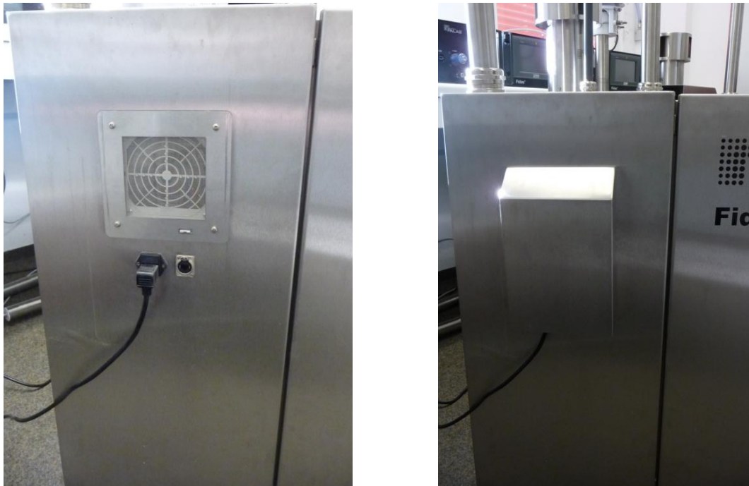
Fig. 23 A+B: Power connection of the weather-protective housing
