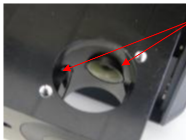
Fig. 34: Optical glasses inside the aerosol sensor
