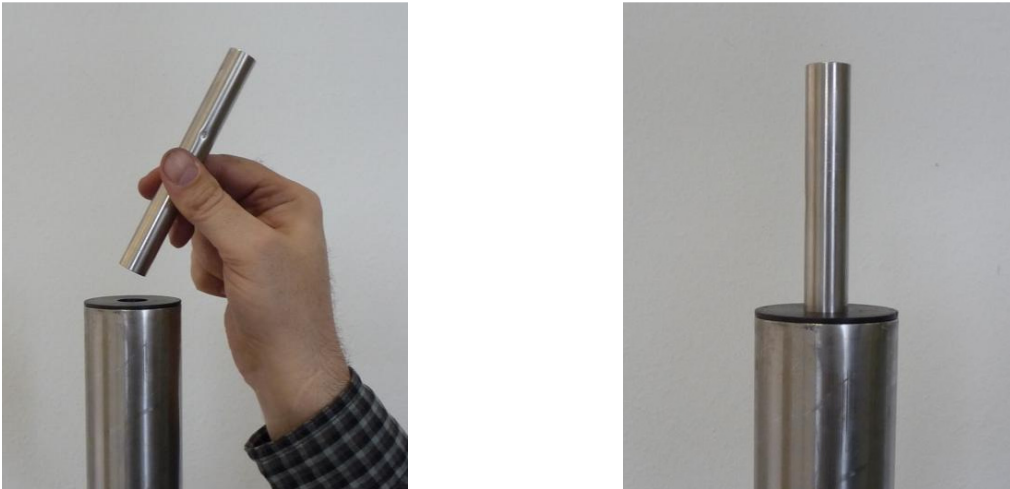
Fig. 21 A+B: Placing of the connection piece
