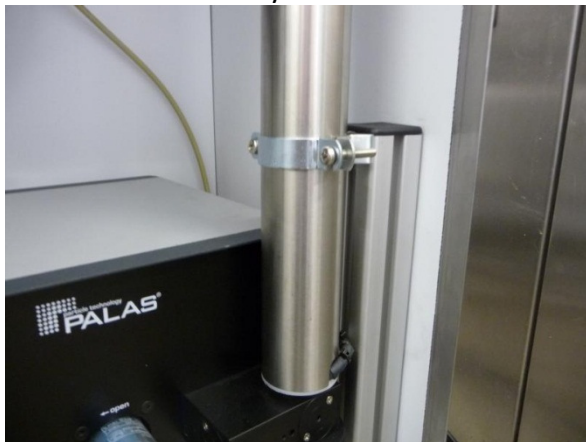
Fig. 19: Internal fixing of the sampling tube
