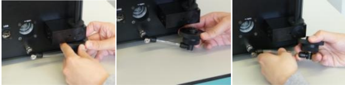
Fig. 28 A-C: Removing the filter holder
