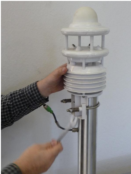
Fig. 9: Mounting of the weather station at the tube
