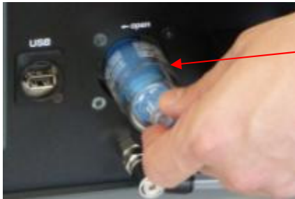
Fig. 36: Removing the protection cap
