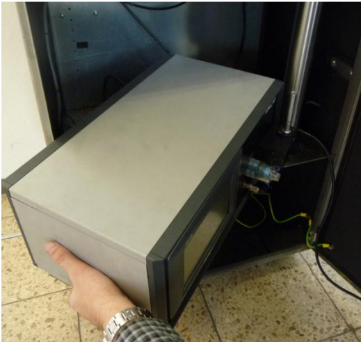
Fig. 15: Insertion of the Fidas® control unit
