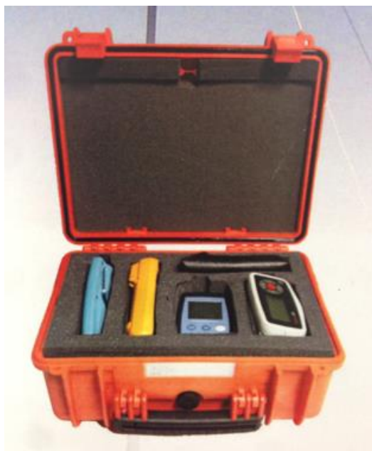
Figure 51 – Air Monitoring Test Equipment Kit (AMTEK) – Customisable
