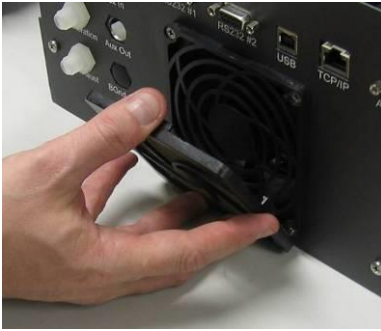
Figure 53 – Removing the Fan Filter
