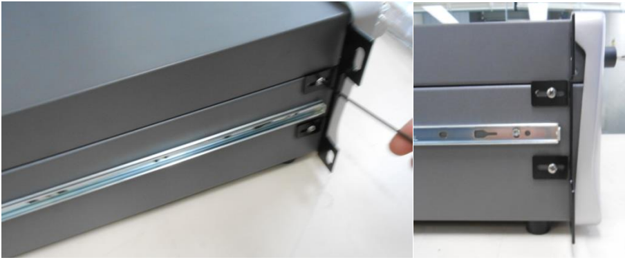
Figure 69 – Rack Mount Ears Fitted to Instrument
