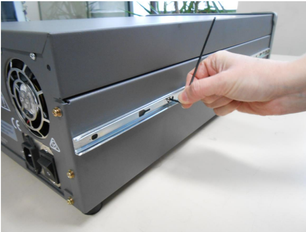
Figure 68 – Assemble Inner Slide on Chassis
