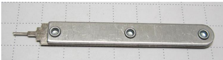
Figure 48 – Minifit Extraction Tool – (T030001)
