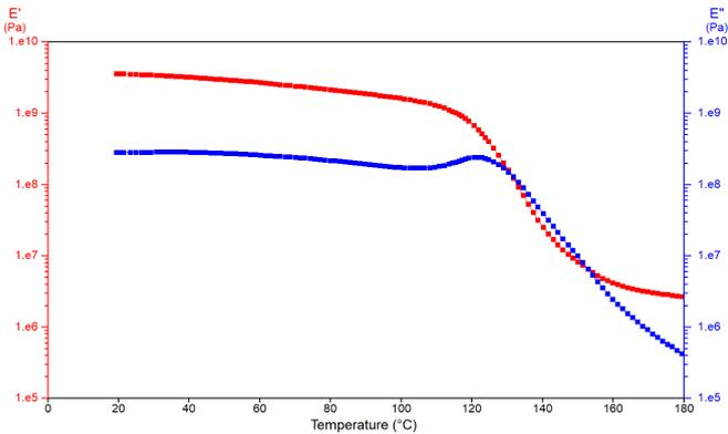
Figure 4. PMMA viscoelastic modulus E' and E'' as a function of the temperature (from 20°C to 180°C) at 1 Hz.
