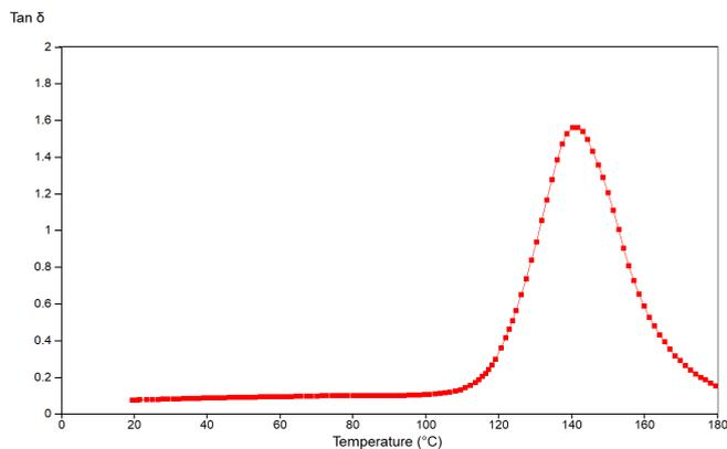
Figure 5. PMMA Tan δ as a function of the temperature (from 20°C to 180°C) at 1 Hz.
