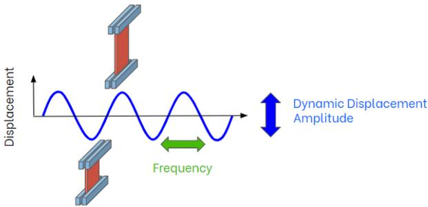
Figure 3. Graphical representation of the dynamic mechanical displacement applied to the specimen
