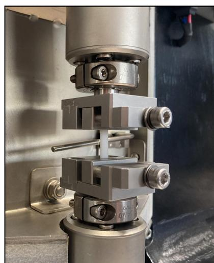
*Figure 2. PMMA specimen fixed between the tension jaw of the specimen holder*
