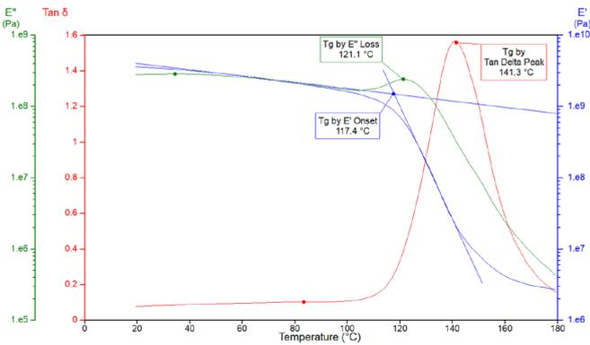
Figure 6. PMMA  $E'$ ,  $E''$  and  $\tan \delta$  as a function of the temperature (from  $20^{\circ}\text{C}$  to  $180^{\circ}\text{C}$ ) at 1 Hz. Different ways to measure the Tg are highlighted.
