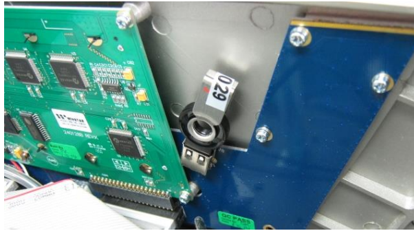
Figure 35 – Installation of USB Memory Stick
