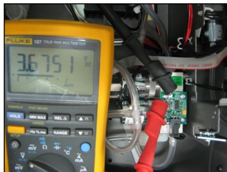
Figure 149 – Typical Test Point Reading of Cell Pressure Sensor
