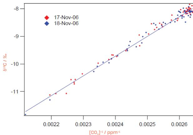
Figure 9. Isotopic ratios can help tracing sources using a Keeling plot. In this case, the intercept of the Keeling plot of δ<sup>13</sup>C vs 1/[CO<sub>2</sub>] is -26.83 ‰, indicative of respiration from the dominant C3 plants in the forest.
