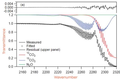
Figure 1. Measured and fitted ambient spectra (lower panel) and residuals associated (upper panel).<sup>1</sup>
