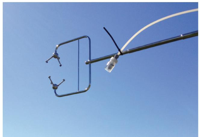
Figure 10. Sonic anemometer for REA measurements.
