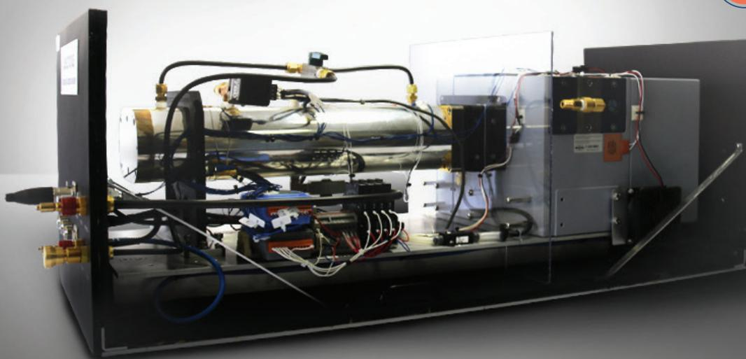
Figure 11. FTIR Spectrometer and measurement cell used in the Spectronus™.
