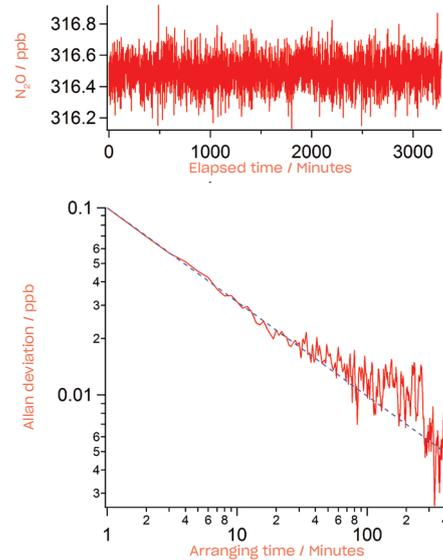
Figure 2. Spectronus™ sensitivity to N<sub>2</sub>O.<sup>1</sup>
