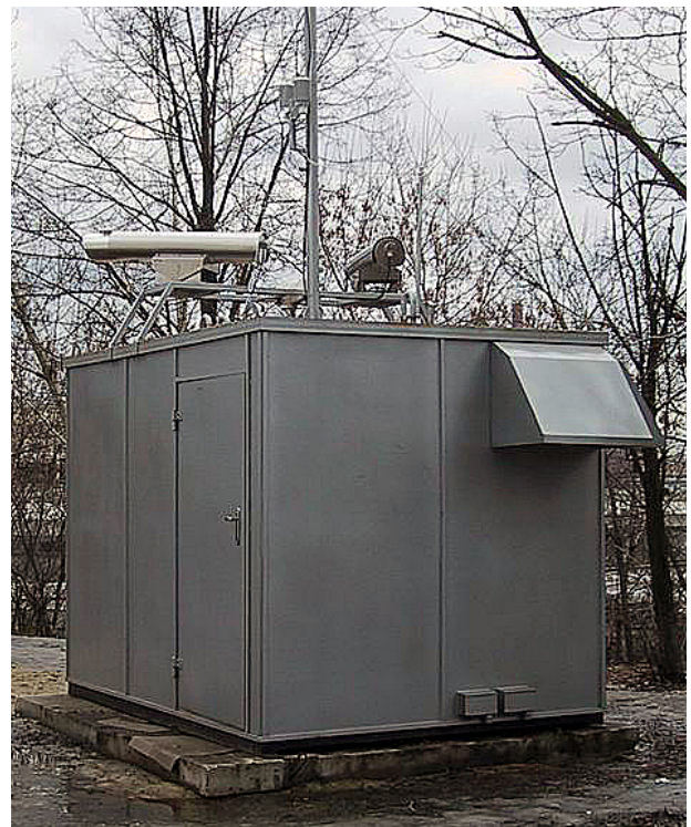
An OPSIS system, mounted on a specially designed moveable container, monitoring the release of air pollutants at street level.
