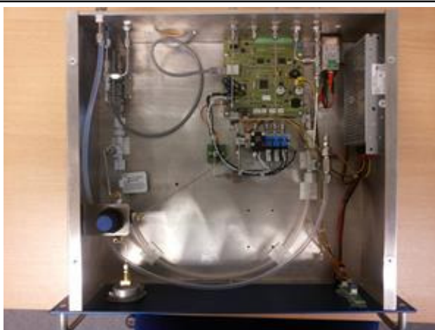
Sample conditioning unit with Perma Pure dryer and humidity sensor
