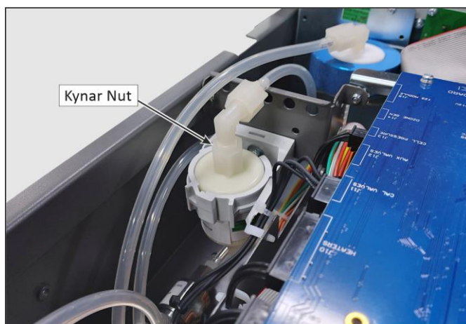
Figure 131 – Remove the Kynar Nut
