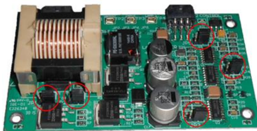
Figure 7 – Lamp Driver PCA Type Jumper Setting (REV D)
