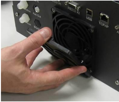
Figure 55 – Removing the Fan Filter
