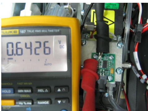
Figure 62 – Typical Test Point Reading of Cell Pressure with Vacuum Connected to Exhaust Port
