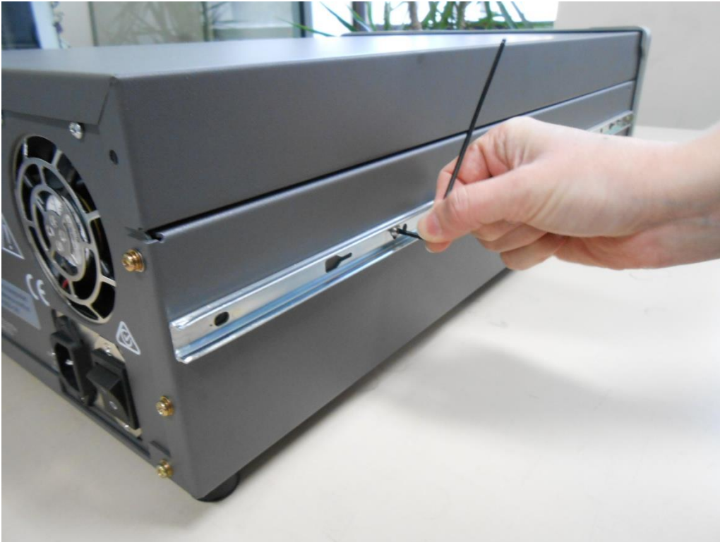
Figure 74 – Assemble Inner Slide on Chassis
