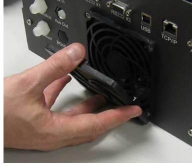
Figure 120 – Removing the Fan Filter
