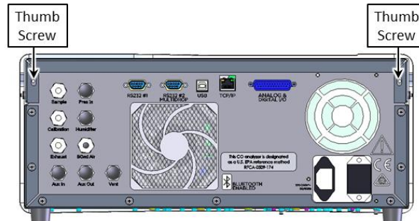
Figure 12 – Opening the Instrument - 1
