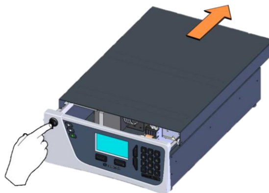
Figure 14 – Opening the Instrument - 3
