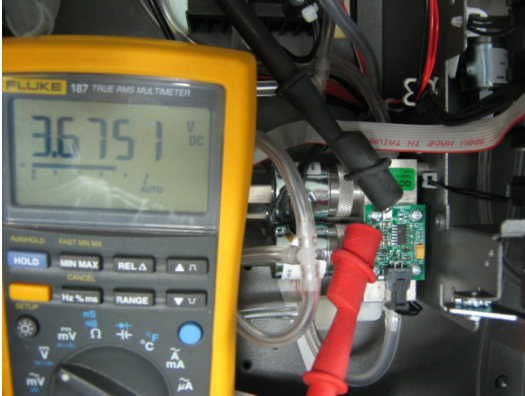
Figure 62 – Typical Test Point Reading of Cell Pressure Sensor
