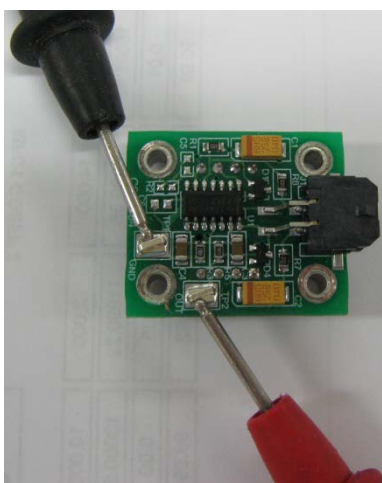
Figure 61 – Test Point Location
