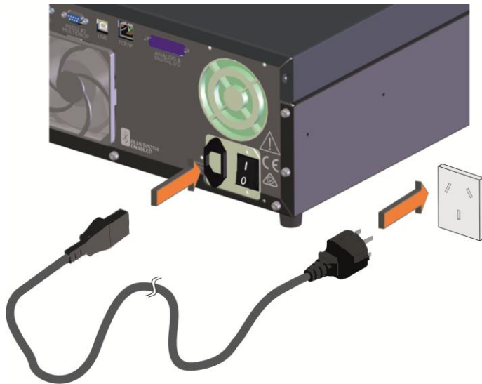
Figure 17 – Connect Power Cord
