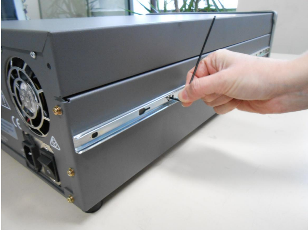
Figure 136 – Assemble Inner Slide on Chassis
