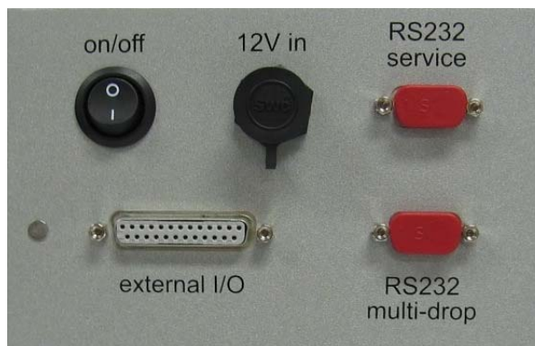
Figure 18 Electrical connections to the Aurora 2000
