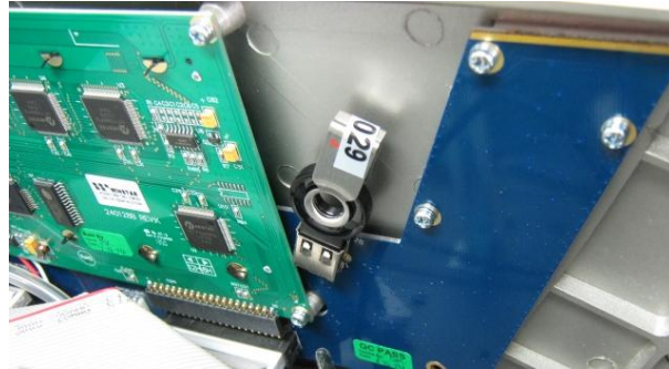
Figure 35 – Installation of USB Memory Stick
