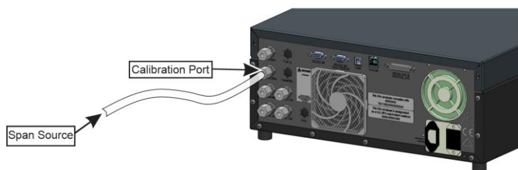
Figure 117 – Span Calibration Set-up - 1
