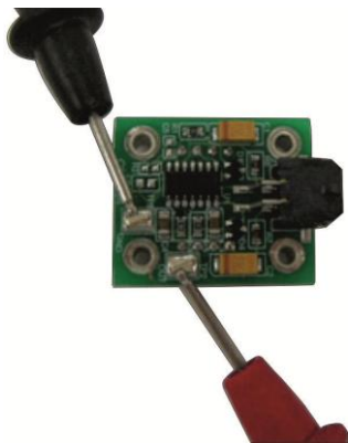
Figure 148 – Test Point Location
