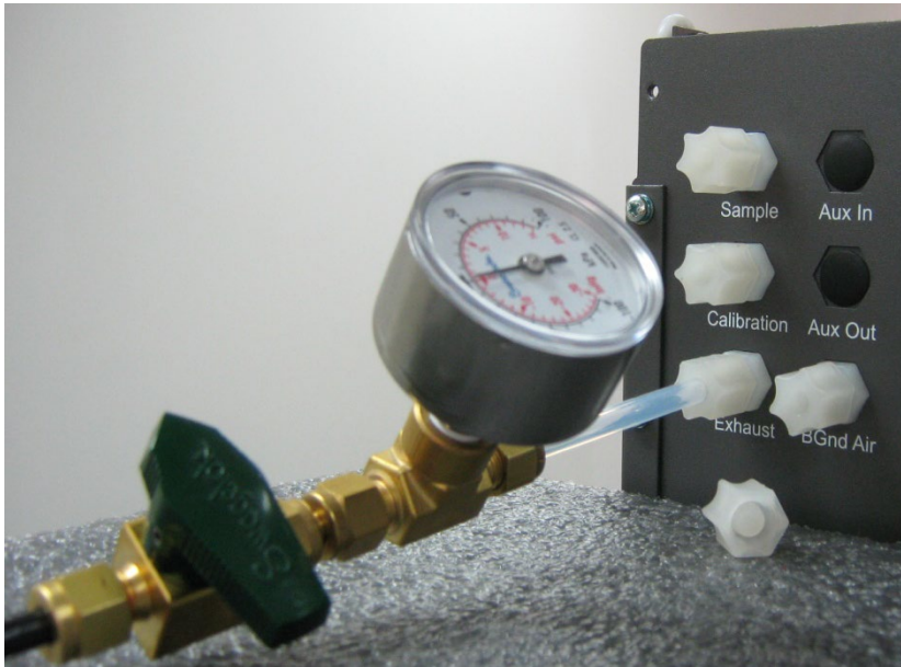
Figure 57 – Leak Test Jig on Exhaust
