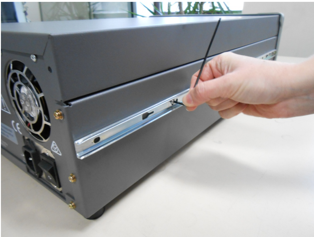
Figure 68 – Assemble Inner Slide on Chassis
