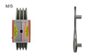
Correct the twist by adding or removing shims on the movable side until the the laser lines are parallel to the center lines.
