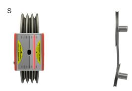
Correct the angle misalignment by rotationg the movable machine horizontally until the laser line (on the stationary side) coincides with the center line.
