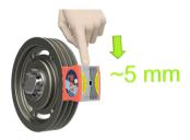
Place the second unit in the opposite groove of the second pulley. Position both units facing each other, and in the corresponding grooves.
