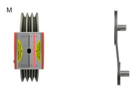
Correct the offset misalignment by moving the movable machine in the axial direction until the laser line (on the movable side) coincides with the center line.
