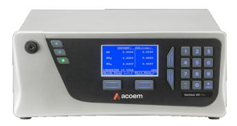
The Serinus® 40 Oxides of Nitrogen (NOx) analyser delivers precise and reliable performance at excellent value. It uses proven chemiluminescence technology to measure NO, NO2 and NOx in ambient air (LDL < 0.4 ppb, range 0 to 20 ppm).
