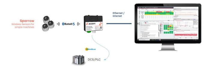
It provides vibration (1 or 3 axis) and temperature measurement. Sensors are easy-to-deploy as it eliminates the wiring for each sensor. Monitored data can be supplied to third party system through Modbus TCP.
