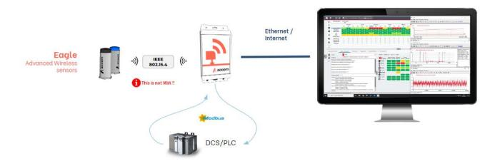
It provides vibration (1 or 3 axis) and temperature measurement. Sensors are easy-to-deploy as it eliminates the wiring for each sensor. Monitored data can be supplied to third party system through Modbus TCP.
