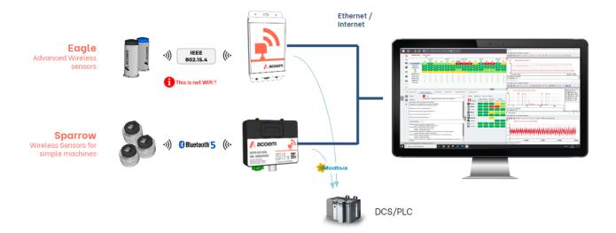
It provides vibration (1 or 3 axis) and temperature measurement. Sensors are easy-to-deploy as it eliminates the wiring for each sensor. Monitored data can be supplied to third party system through Modbus TCP.
