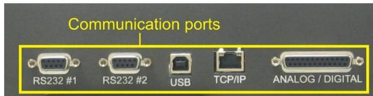
Figure 11 Communication ports
