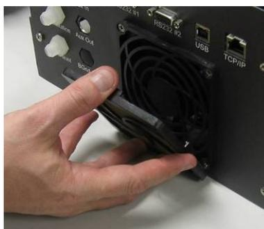
Figure 19 Removing fan filter
