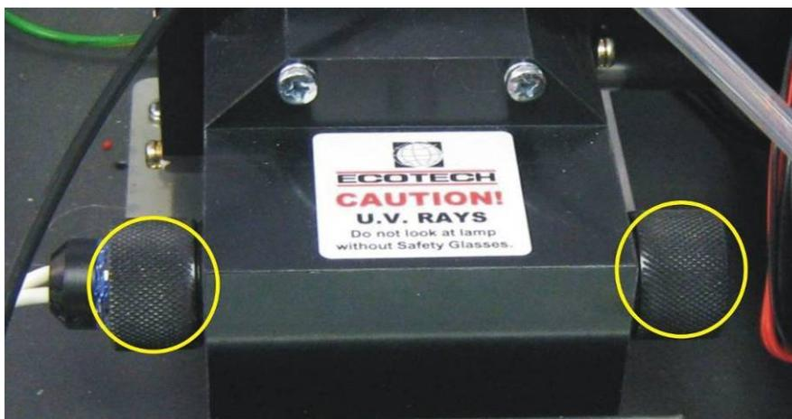
**Figure 23 Collets of the UV lamp**
