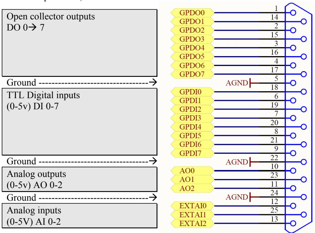
Figure 12 External 25pin I/O individual pin descriptions
