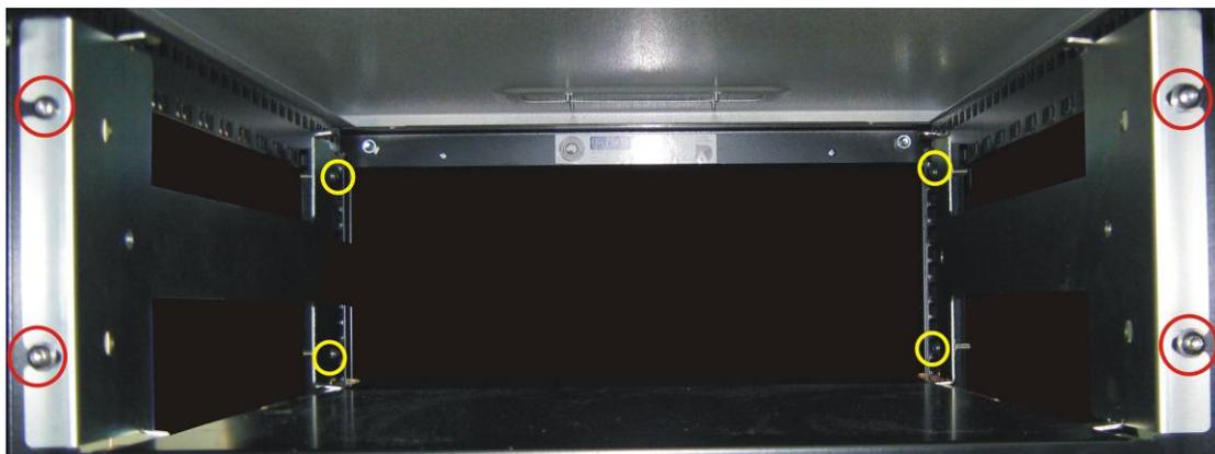
Figure 25 Installation of rack mount brackets
