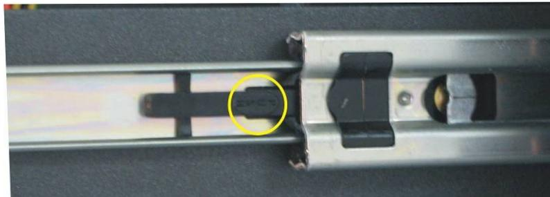
**Figure 27 Rack slide lock**
