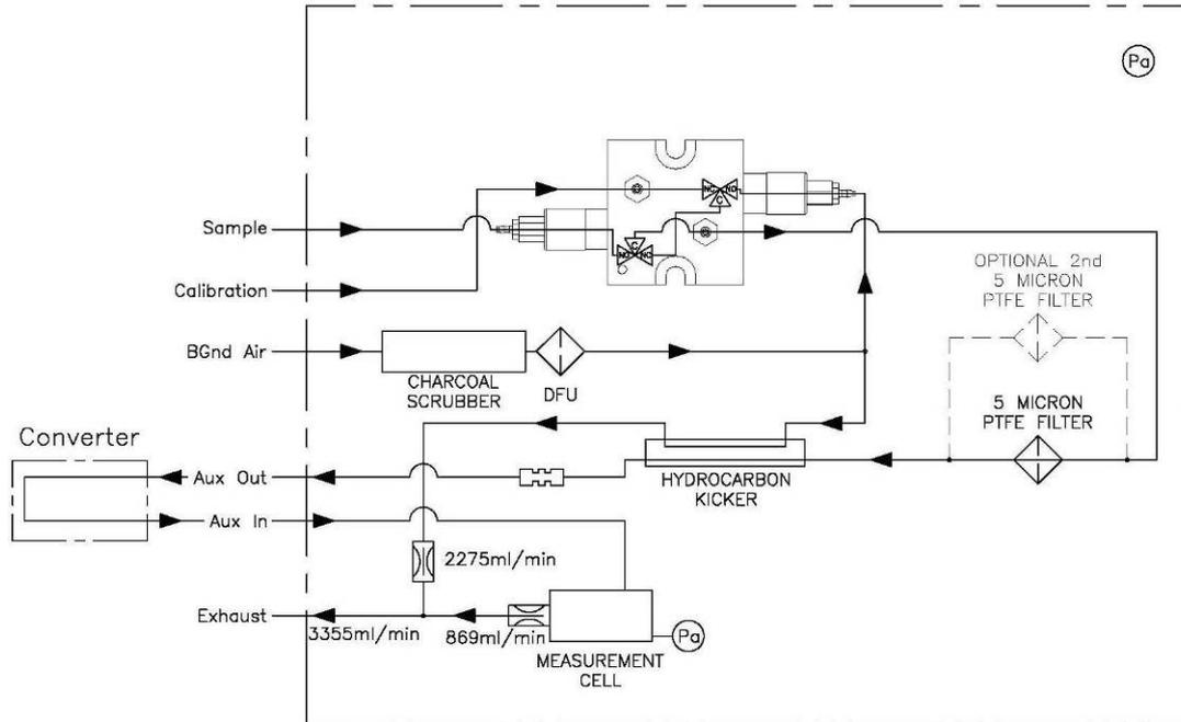
Figure 17 Pneumatic diagram
