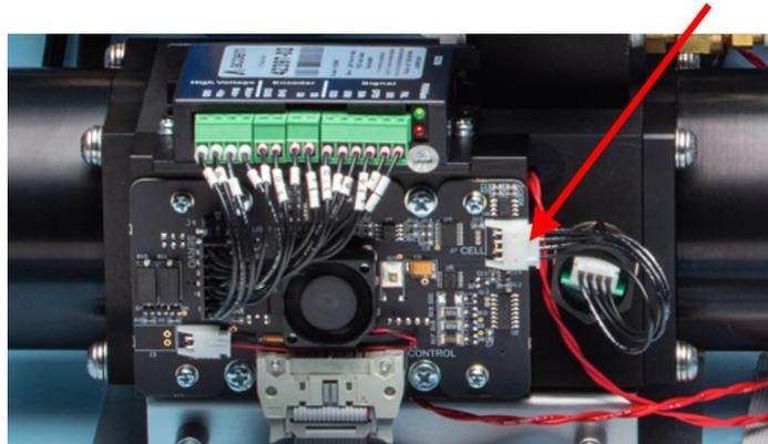
**Figure 180 – Location of Pressure, Temperature and Relative Humidity Sensor Cable**
