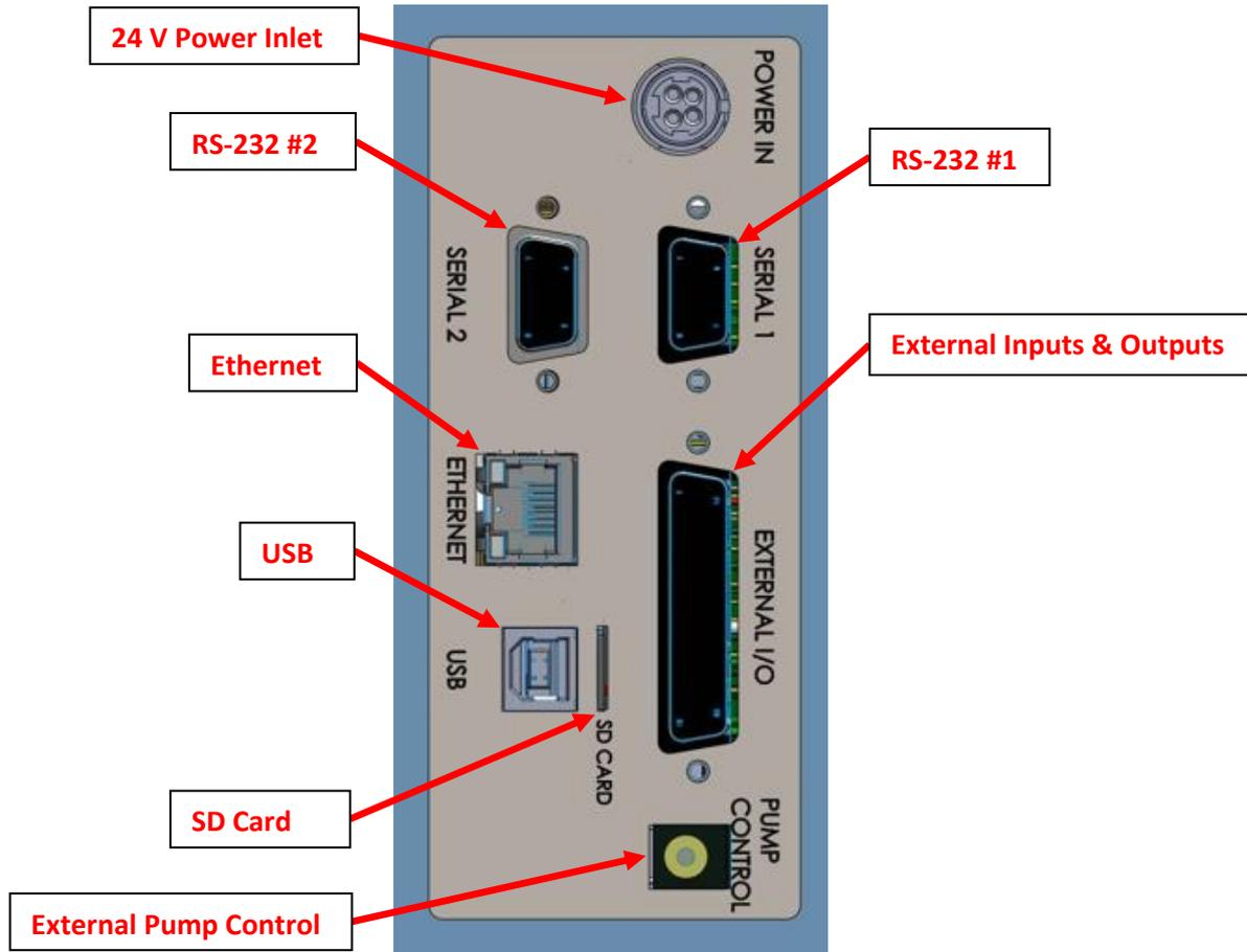
Figure 29 – Power and Communication Panel Diagram
