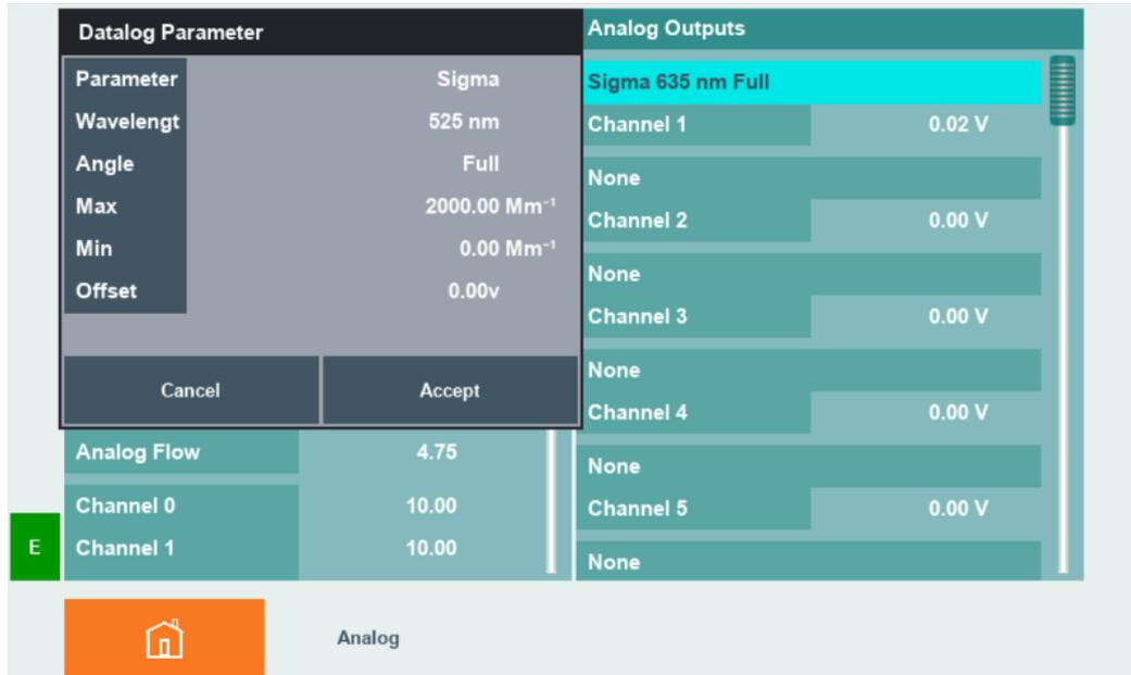
**Figure 110 – Analog Outputs Setup Panel**
