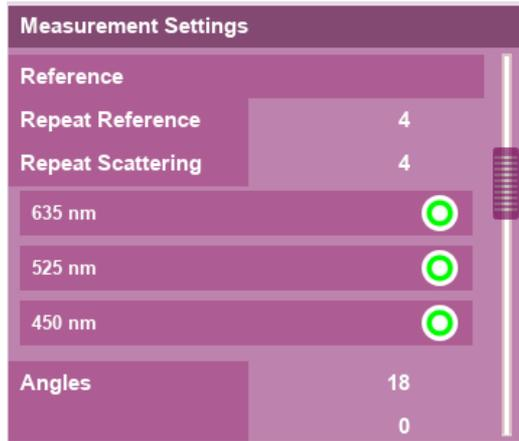
**Figure 217 – Example of NE-400 Wavelength Selection**
