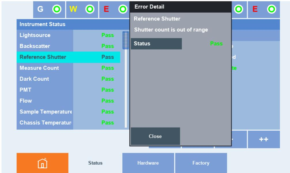
**Figure 130 – Instrument Status Popup Dialog Box for Error Detail**
