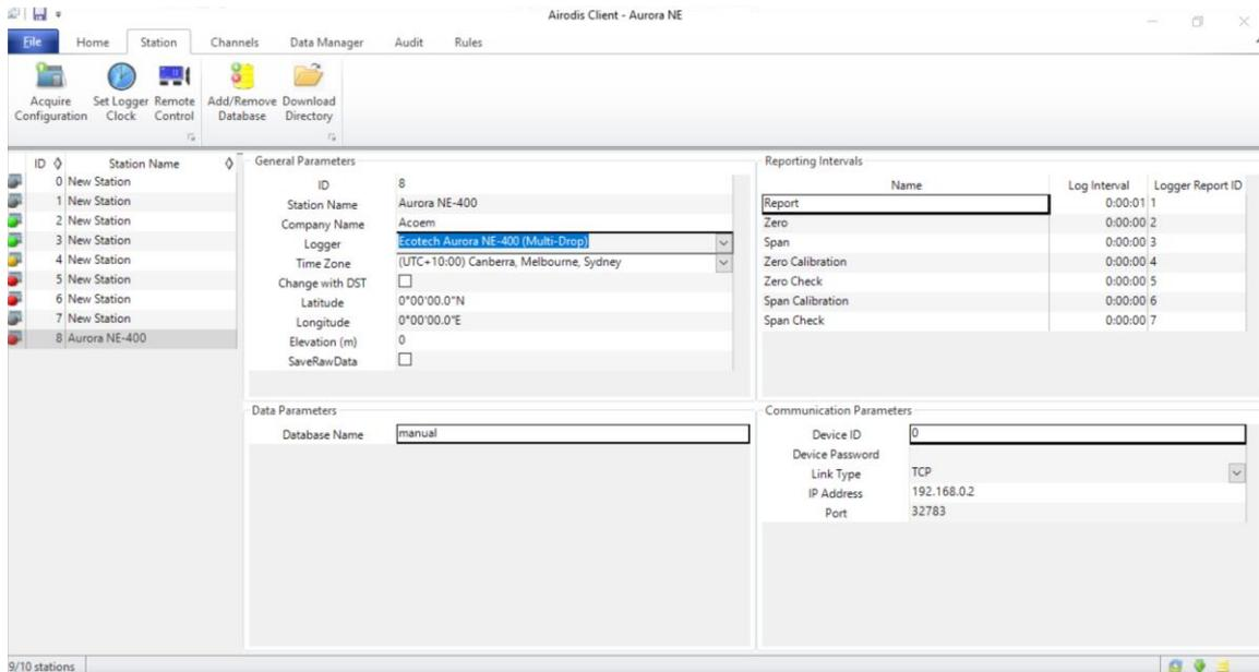
Figure 154 – LAN Network Set-Up (Airodis)
