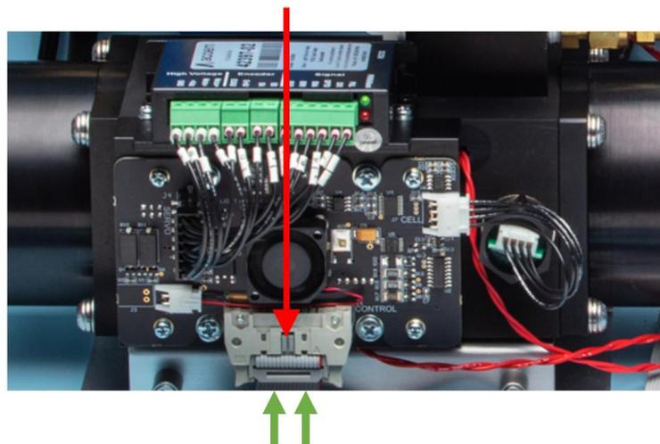
**Figure 184 – Connecting Light Source Ribbon Cable**
