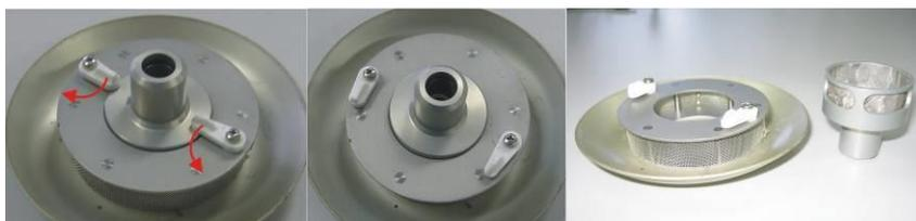
**Figure 176 – Sample Inlet Cleaning**
