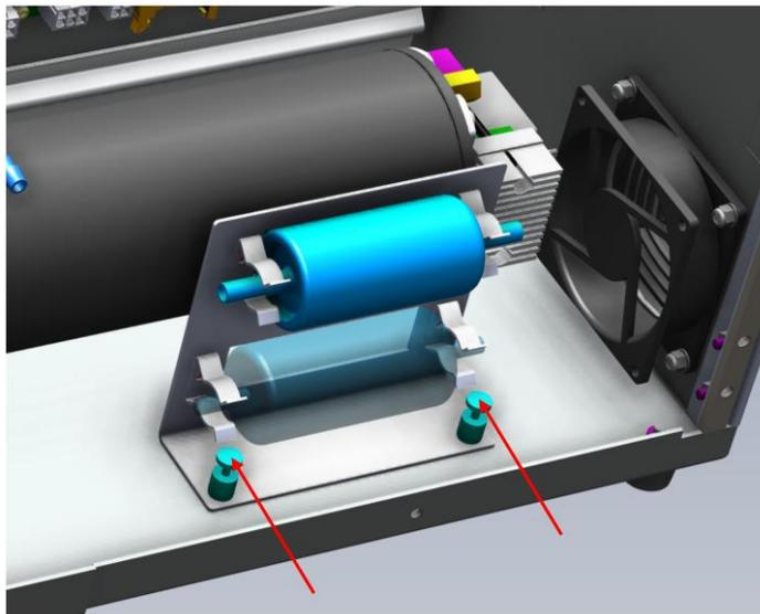
**Figure 187 – Filter Holder Captive Screw Location**
