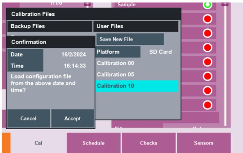
Figure 74 – Calibration Configuration Load Confirmation
