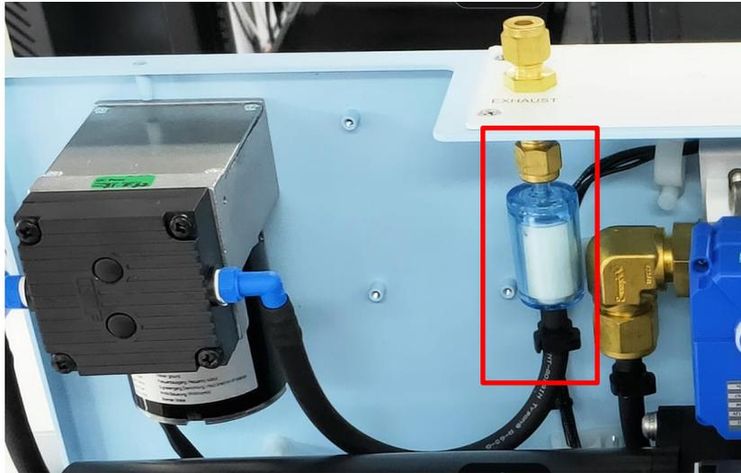
**Figure 177 – Pump Filter**
