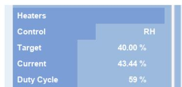
**Figure 137 – Heater Control Set To RH**
