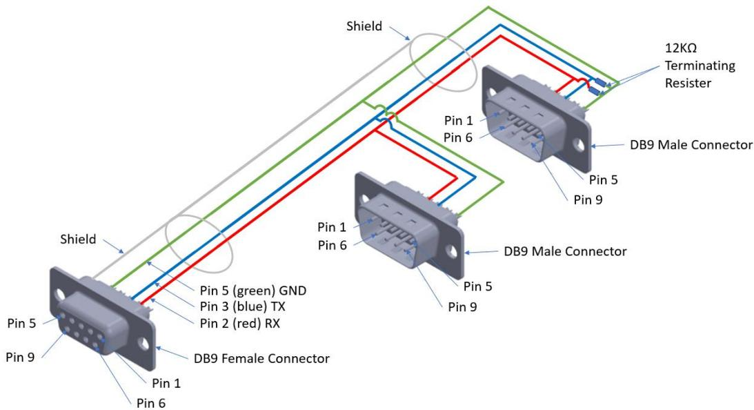
**Figure 149 – RS-232 Multidrop Cable Example**
