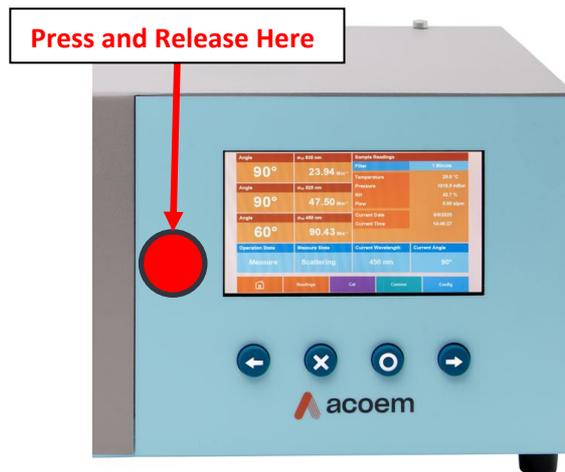
**Figure 32 – Front Door Release Location**
