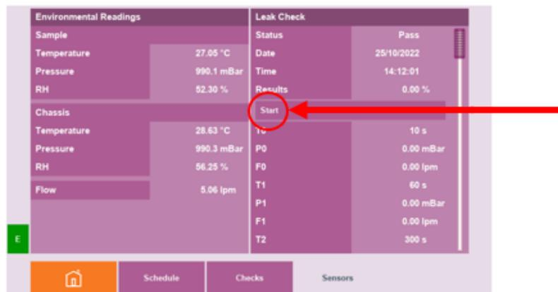
**Figure 208 – Location of Leak Check Start Button**
