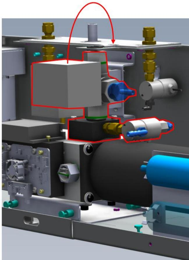
**Figure 190 – Placement of Sample Manifold Assembly**
