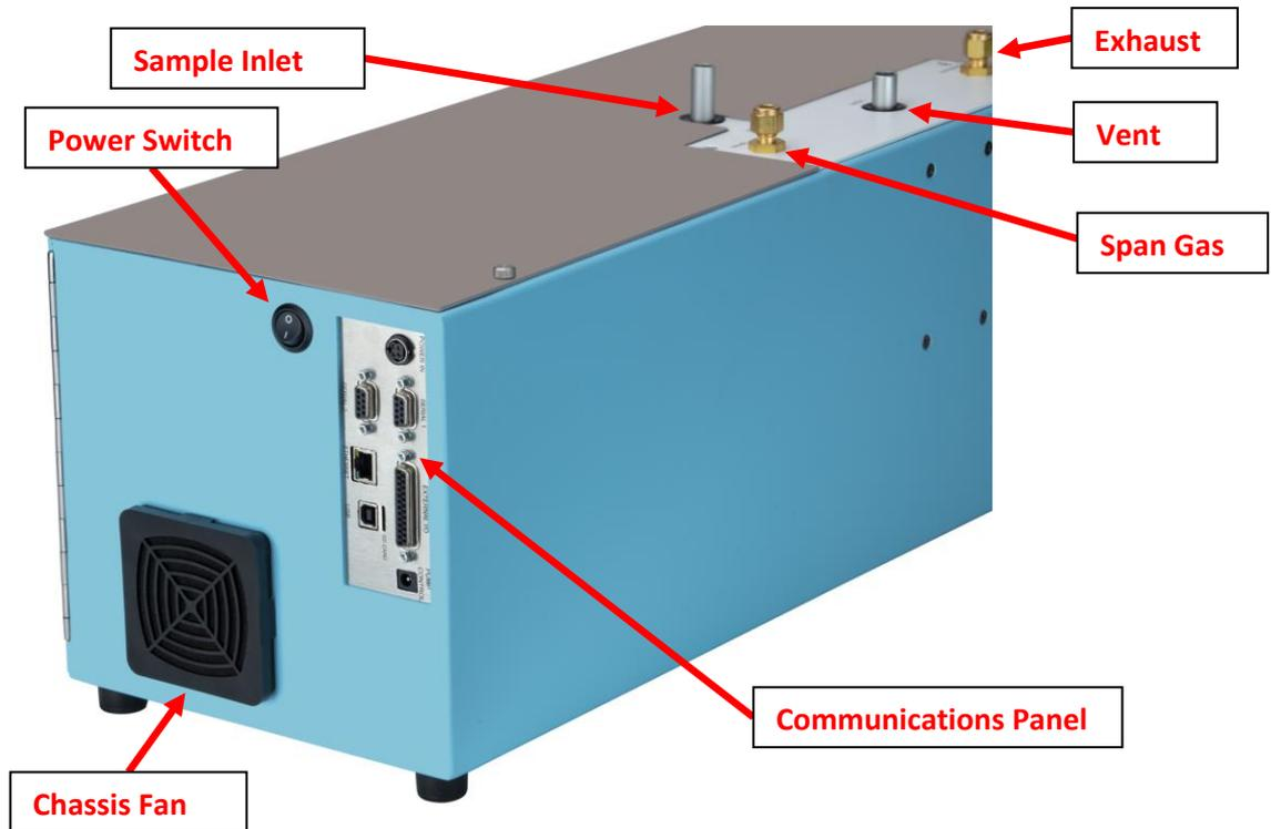
Figure 28 – External Connections Diagram
