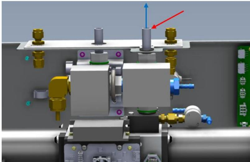
**Figure 186 – Sample Inlet Tube Location**
