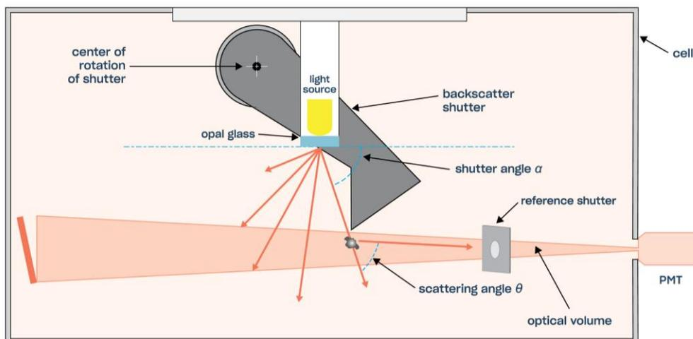
Figure 6 – Light Path, With 90° Backscatter
