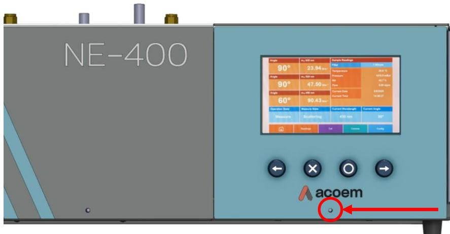
**Figure 31 – Transit Thumb Screw Location**
