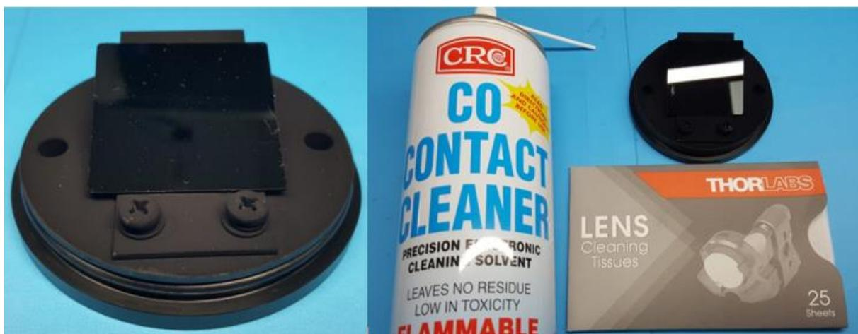
**Figure 201 – Light Trap Mirror Cleaning**
