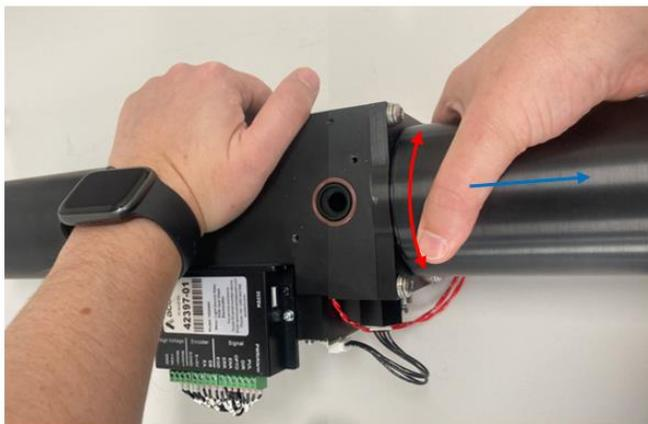
Seal broken stop at this point
