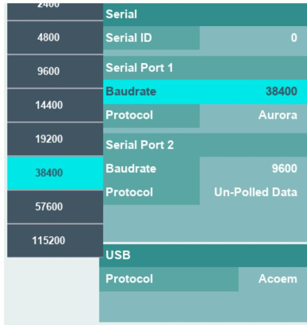
**Figure 105 – Serial Panel Baudrate selection**
