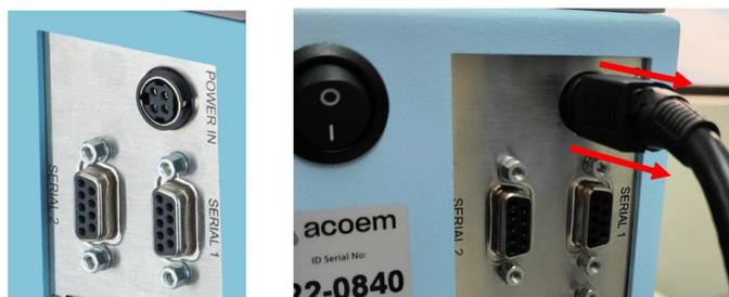
Figure 40 – Power Connector removal
