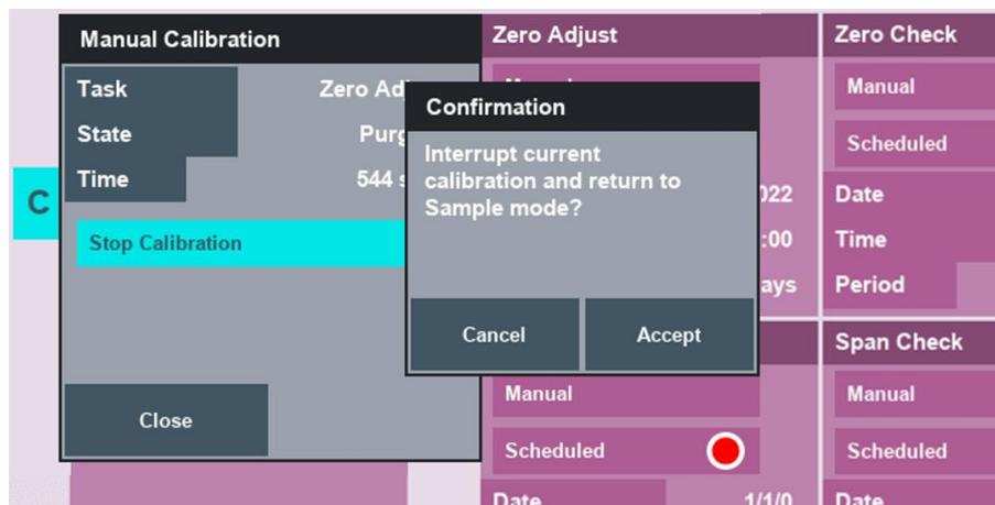
**Figure 83 – Stop Calibration Confirmation Dialog Box**
