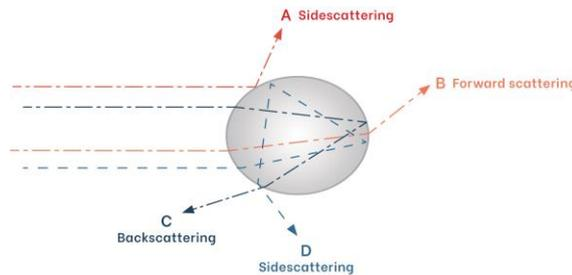
**Figure 2 – Light Scattering and Absorption**
