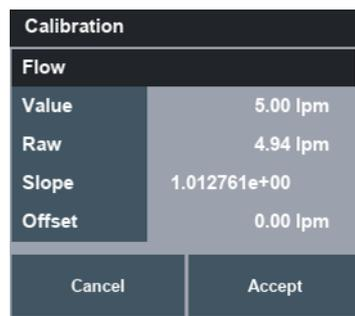
**Figure 167 – Flow Calibration Slope and Offset**
