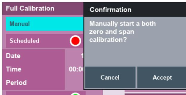
Figure 77 – Manual Full Calibration Confirmation Dialog Box
