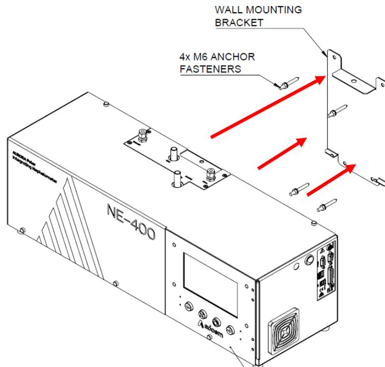
**Figure 39 – Wall Mount Bracket Installation Step 3**
