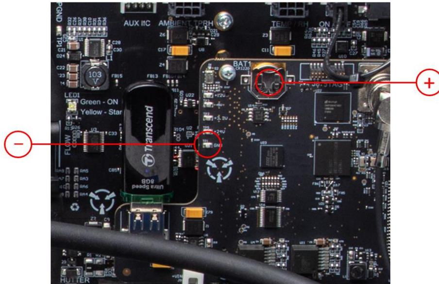
**Figure 218 – Polarity of Clock Battery Test Points**
