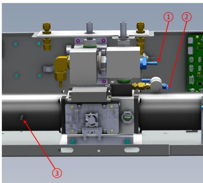
**Figure 207 – Reconnecting Tubing**
