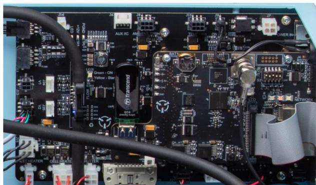
Figure 27 – Microprocessor PCA and Control PCA
