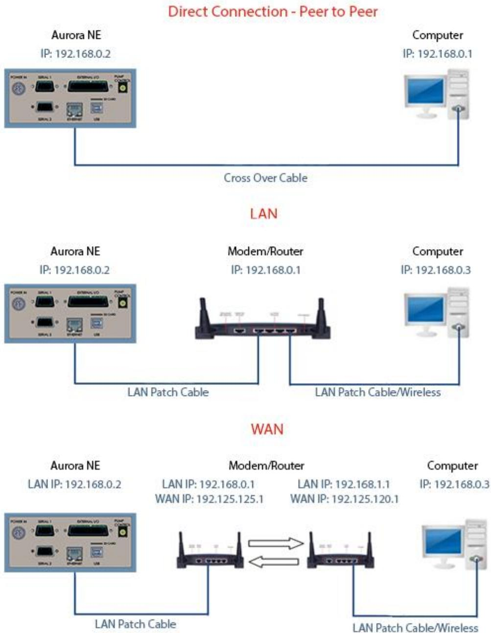
**Figure 152 – Example of Typical Network Setups**
