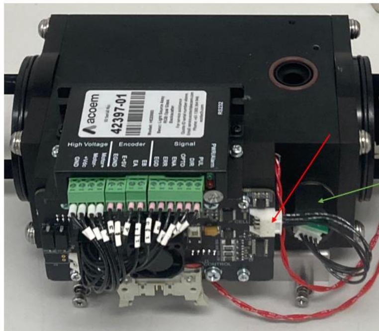
**Figure 198 – Location of TPRH Sensor and Cable**
