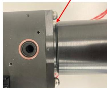
**Figure 195 – Tube Casing Removal – PMT End**
