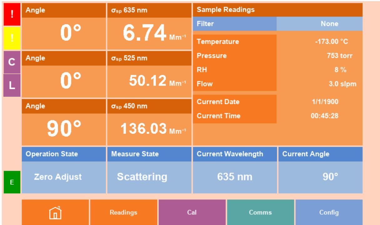
Figure 43 – Example - Colour Touch Screen for an Aurora NE-400
