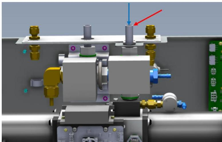
**Figure 206 – Replacing Sample Inlet Tube**
