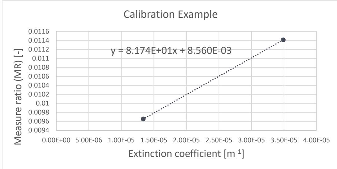
**Figure 13 – Aurora NE Calibration Curve**
