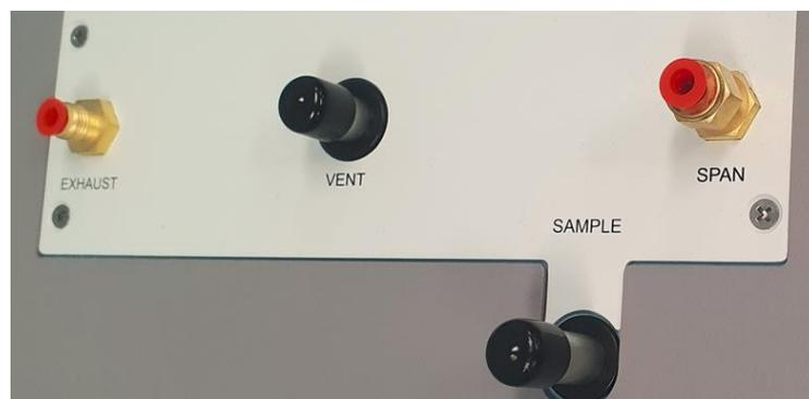
**Figure 42 – Pneumatic Ports Plugged and Capped**
