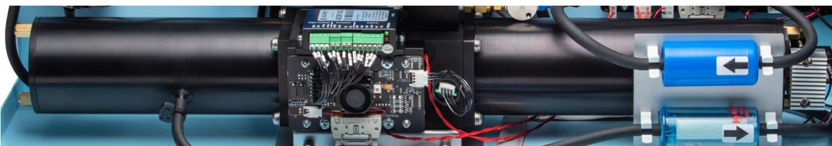
Figure 17 – NE-300 Measurement Cell assembly
