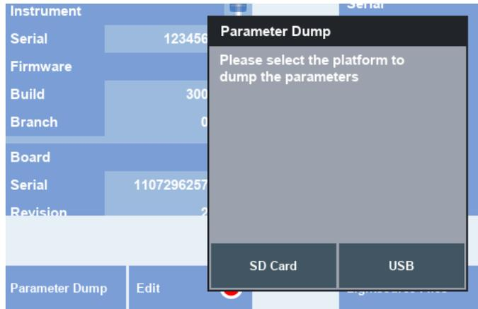
**Figure 146 – Parameter Dump Storage Location Selection**
