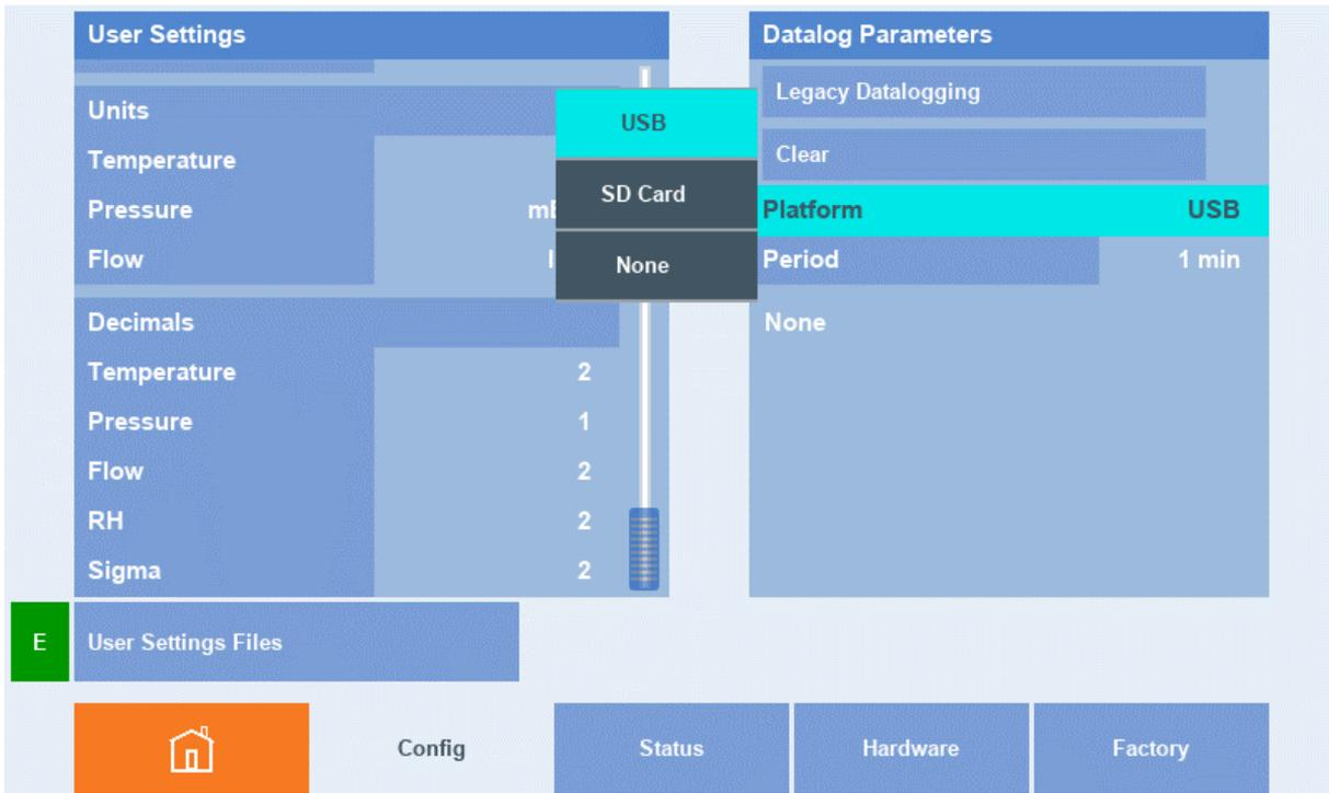
Figure 157 – Data Logger Storage Location
