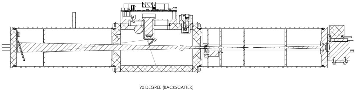
**Figure 18 – NE-300 Measurement Cell cross section**
