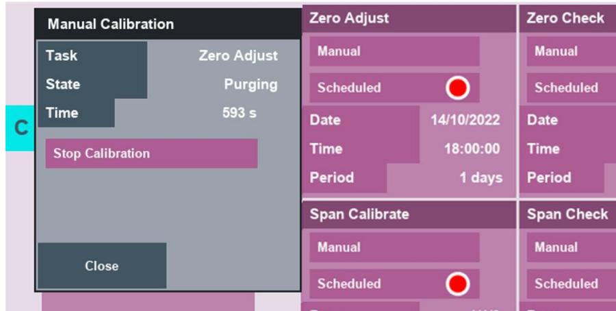
**Figure 82 – Manual Calibration Dialog Box**
