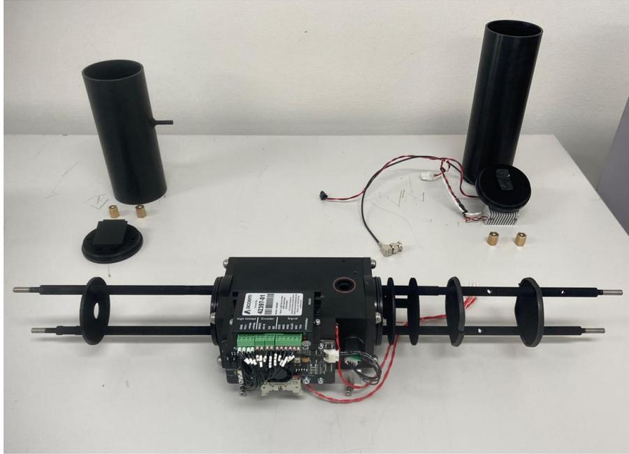
**Figure 197 – Endplates and Tube Casings Removed**
