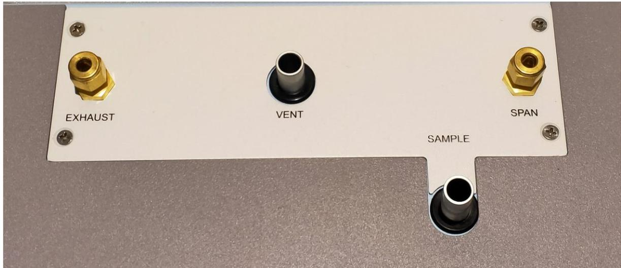
Figure 41 – Pneumatic Ports
