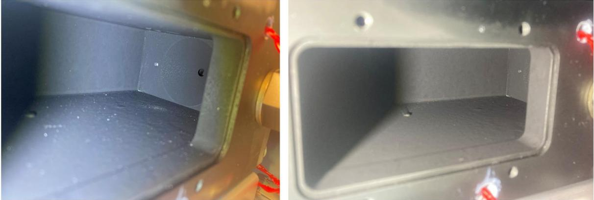
**Figure 183 – Cell Body Clean Before and After**
