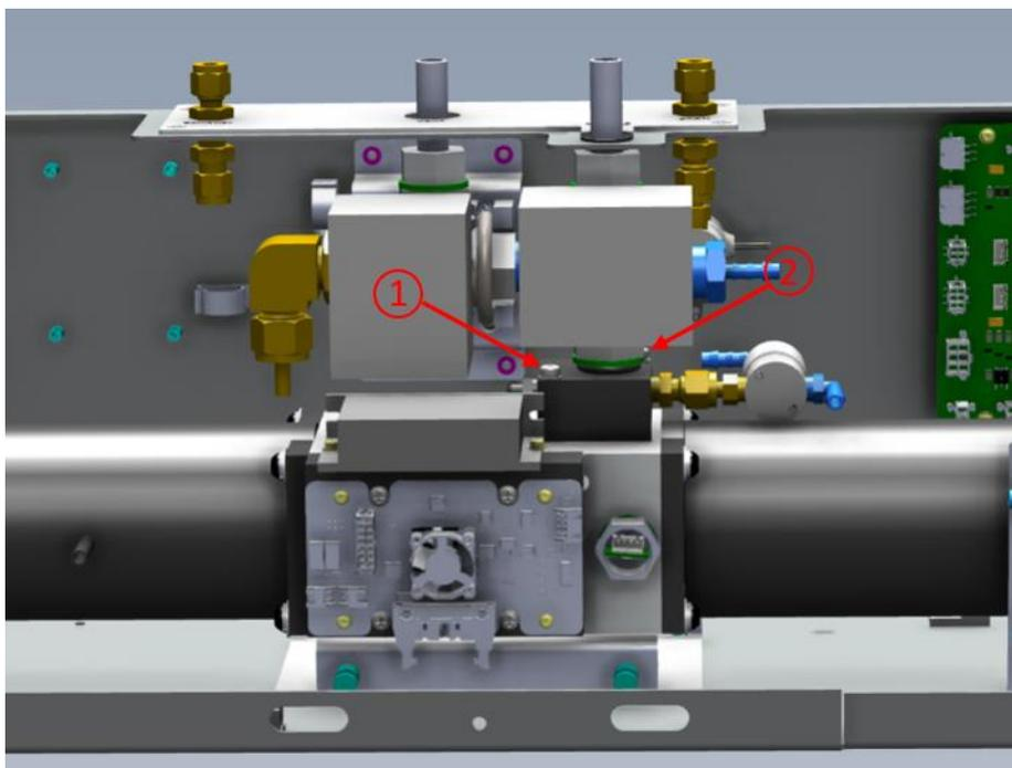
**Figure 189 – Location of Sample Manifold Screws**
