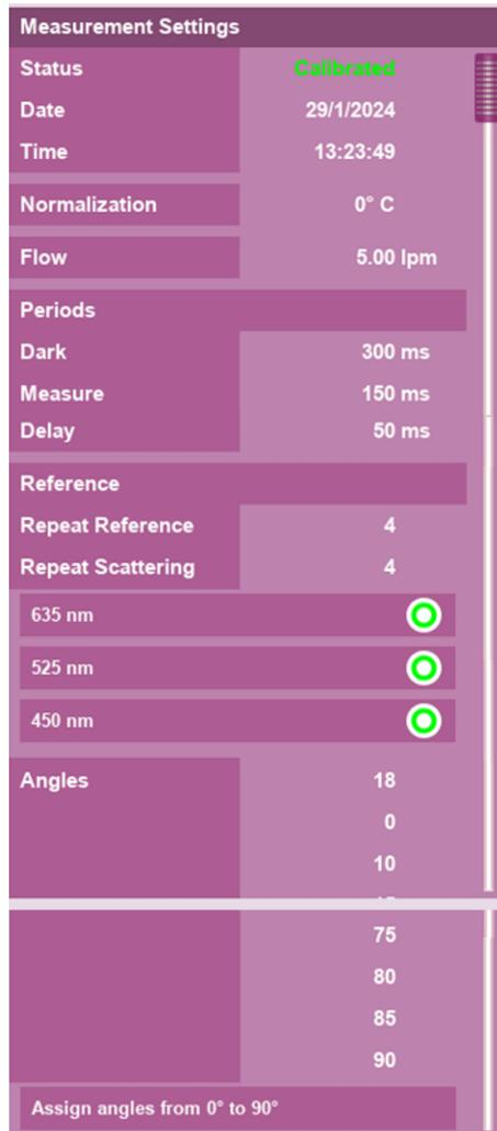
**Figure 60 – Measurement Settings Panel NE-400 (Service Menu enabled)**
