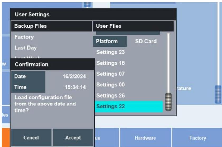
**Figure 127 – User Settings Configuration Load Confirmation**
