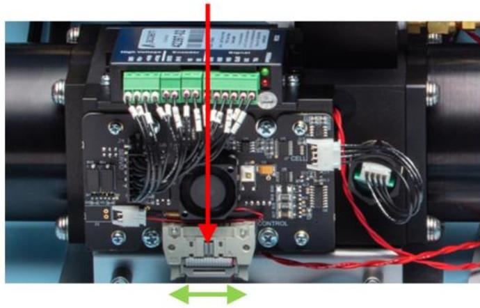
**Figure 179 – Ejecting Light Source Ribbon Cable**
