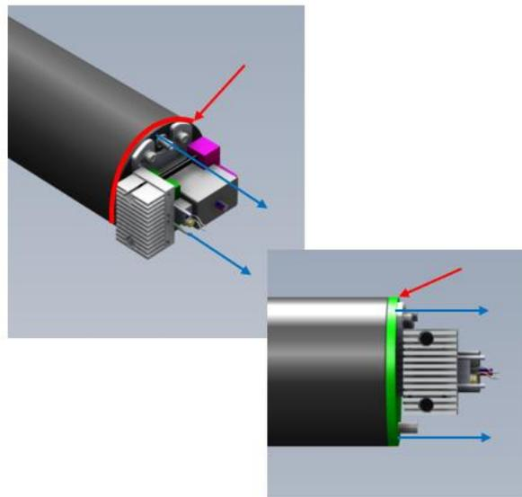
Figure 193 – PMT Endplate Removal
