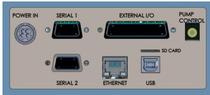
Figure 148 – Communication Ports
