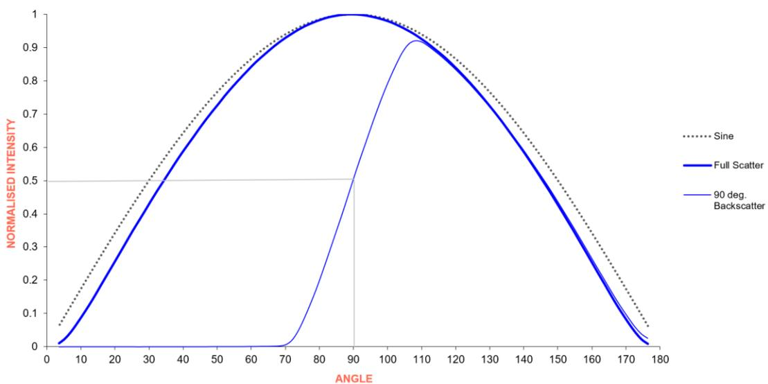
Figure 8 – Backscatter Light source Distribution (90°)
