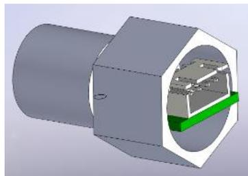
**Figure 25 – Sample Temperature/Pressure/RH Sensor**
