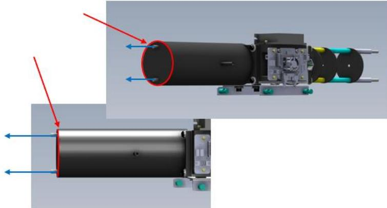
**Figure 196 – Light Trap Endplate Removal**
