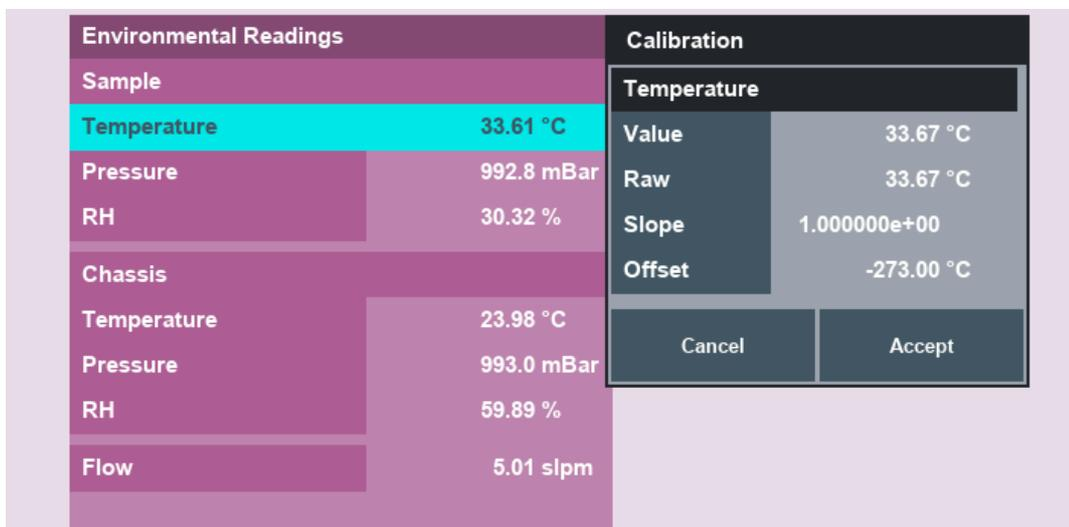
**Figure 100 – Sample Temperature Calibration Dialog Box**
