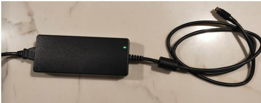
Figure 16 – 24 VDC Power Supply
