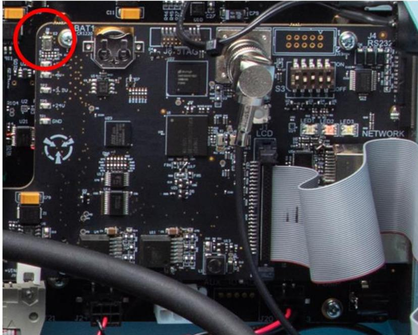
Figure 164 – Location of The Chassis Temperature Pressure RH Sensor
