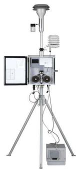
The E-BAM Plus is a portable, real-time beta gauge built to satisfy users, regulators and those from the health community by providing truly accurate, precise and automatic measurement of fine particulate matter. (Accuracy exceeds US EPA PM<sub>10</sub> FEM requirements, range 0 to 10 mg/m<sup>3</sup>.)
