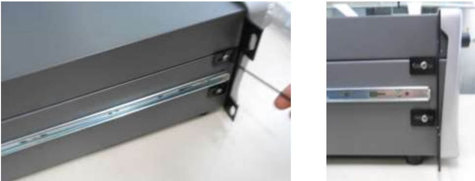
Figure 99 – Rack Mount Ears Fitted to Analyser
