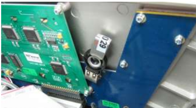
Figure 16 – Installation of USB Memory Stick
