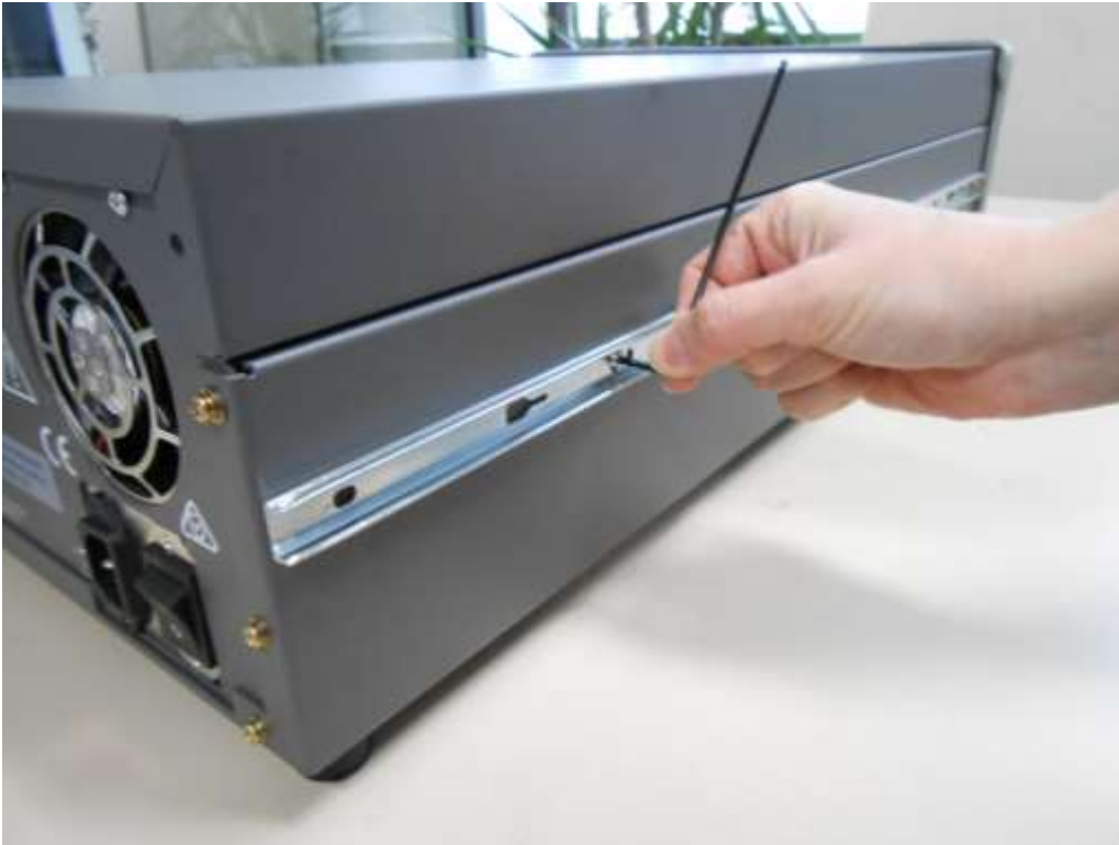
Figure 98 – Assemble Inner Slide on Chassis
