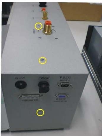
Figure 53 – Pump bracket screws
