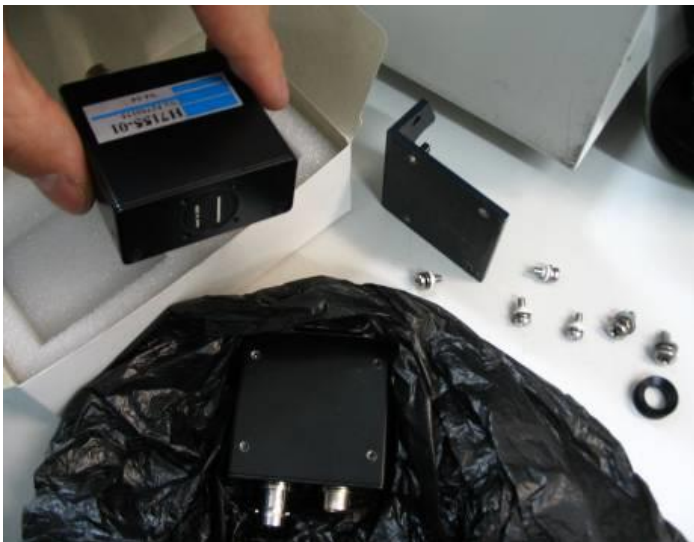
Figure 50 – New PMT inserted
