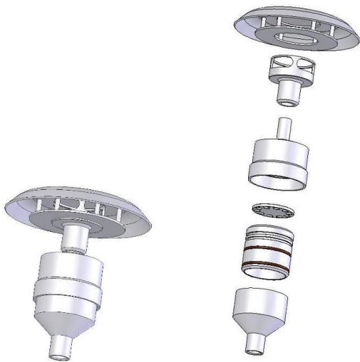
Figure 57 – PM 2.5 inlet collapsed and expanded
