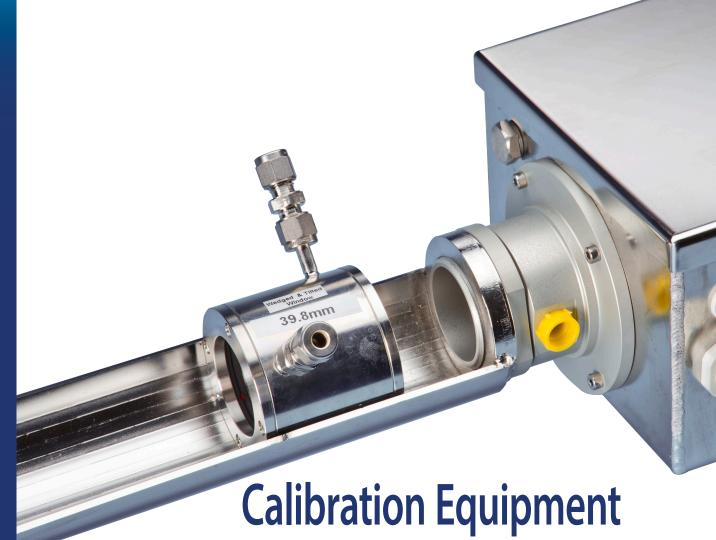
OPSIS offers a range of calibration equipment for use with its continuous emissions monitoring systems. The following equipment is used for manual calibration of systems based on ER060. It is based on the CB100 calibration bench. This is used with an EM060 light emitter at one end and an RE060 receiver at the other, with the receiver being connected to the analyser by a fibre optic cable. The set-up creates a light path for manual calibration.
