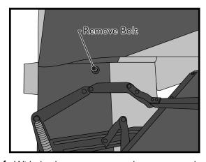
**4.** With the dustcover open, you have access to the bolt securing the arm to the back. Remove the bolt, as shown in the figure above, from both sides of the comfort sleeper.
