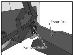
**9.** Remove the two bolts on each side of the comfort sleeper that secure the front rail to the arm. With the bolts removed, set the front rail aside.
