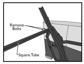
**8.** To remove the square tube, remove the two bolts on both sides of the comfort sleeper. With all (4) four bolts removed, set the square tube aside.
