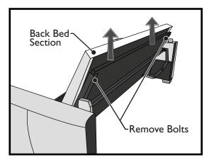
**7.** Remove (4) four bolts on each side of the comfort sleeper that secure the back bed section to the mechanism. Start from the bottom, leaving a single top bolt on each side. Hold the back bed section while removing the last two bolts. Set the back bed section aside.
