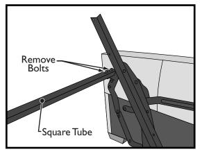
**7.** To remove the square tube, remove the two bolts on both sides of the comfort sleeper. With all (4) four bolts removed, set the square tube aside.
