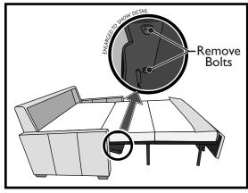
**I.** To begin, open the comfort sleeper as shown. Remove the two bolts connecting the middle bed section to the mechanism, as shown in the enlarged view. Do this on both the left and right sides.
