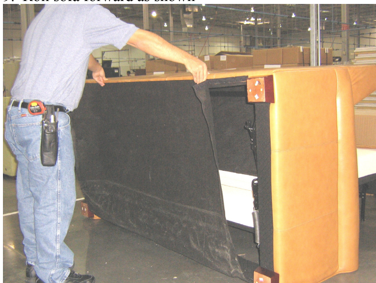
11. Position hands in a wide stance and attach dustcover being careful not to create diagonal wrinkles
