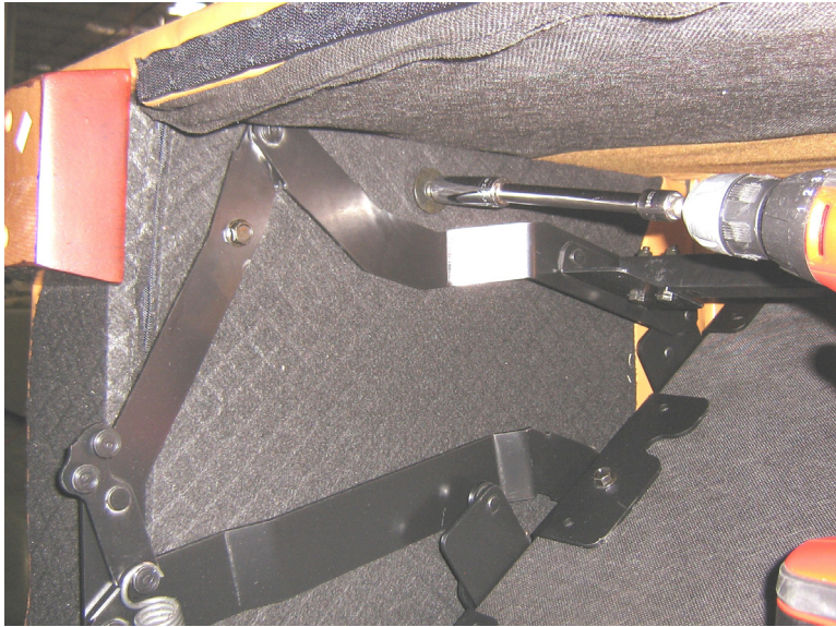
3. Remove bolt(s) on each side of sofa as shown. Sofas where the Back of the sofa does not overhang the Arm have more than one bolt on each side of the sofa
