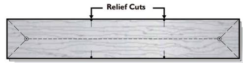
2. Using a concave knife / a utility blade knife / a saw (set saw depth to board thickness) cut along lines and remove center section. Make relief cuts using drilled holes as visible stop.
