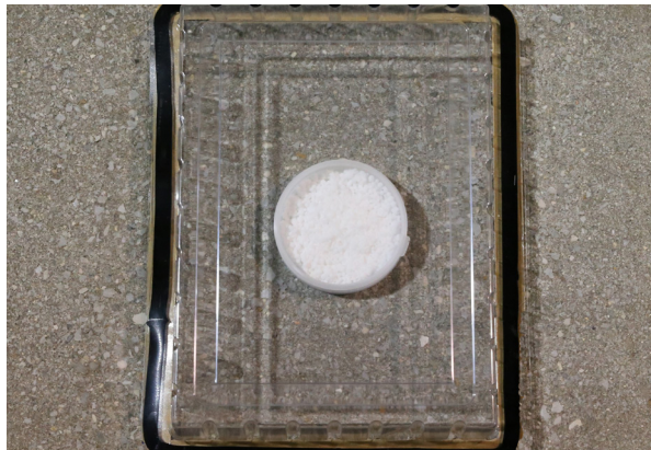
Calcium Chloride Test (ASTM F1869) This test method allows you to obtain a quantitative value indicating the moisture vapor emissions rate (MVER) from the surface of a concrete subfloor using
