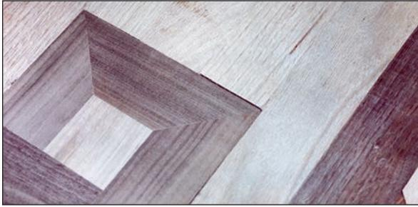
The best way to disguise a gap between boards such as the one against the French knot above is to use the slivering technique.
