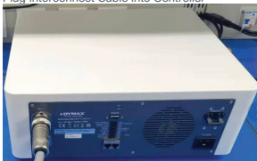
Figure 12. Plug Interconnect Cable into Controller
