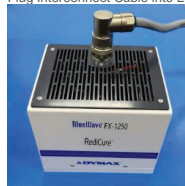
Figure 13. Plug Interconnect Cable into Emitter
