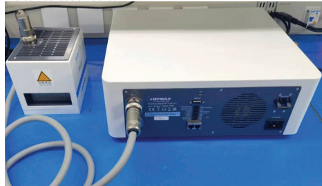
Figure 7. Interconnect Cable Installed
